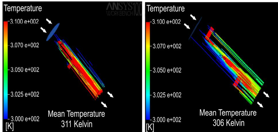
Fig. 2. Water-Air Heating  $6\text{m}^3/\text{h}$  and  $12\text{m}^3/\text{h}$
