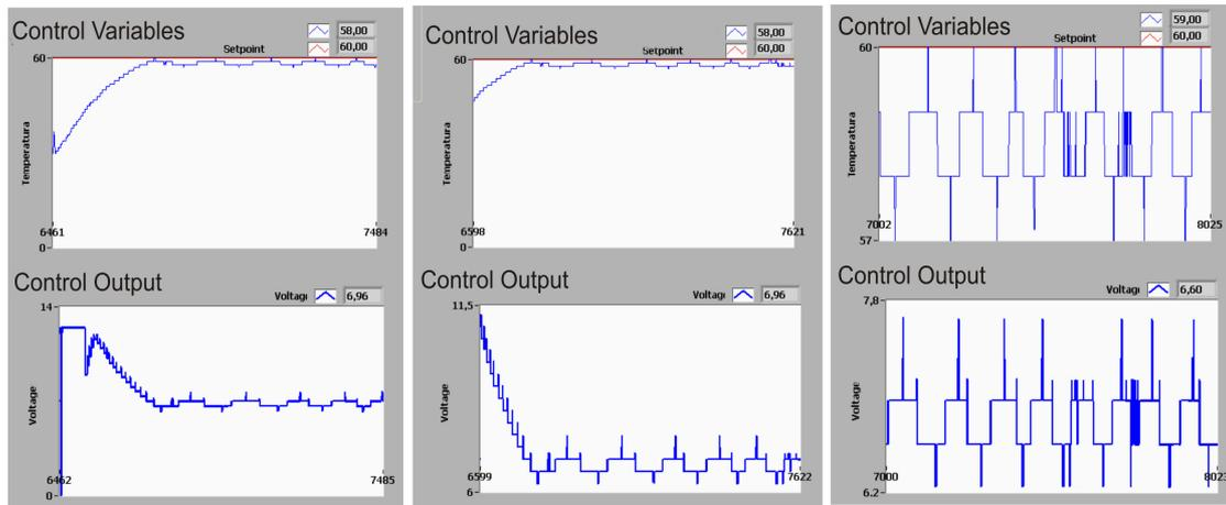
Fig. 7. Process the Fuzzy-PID control
