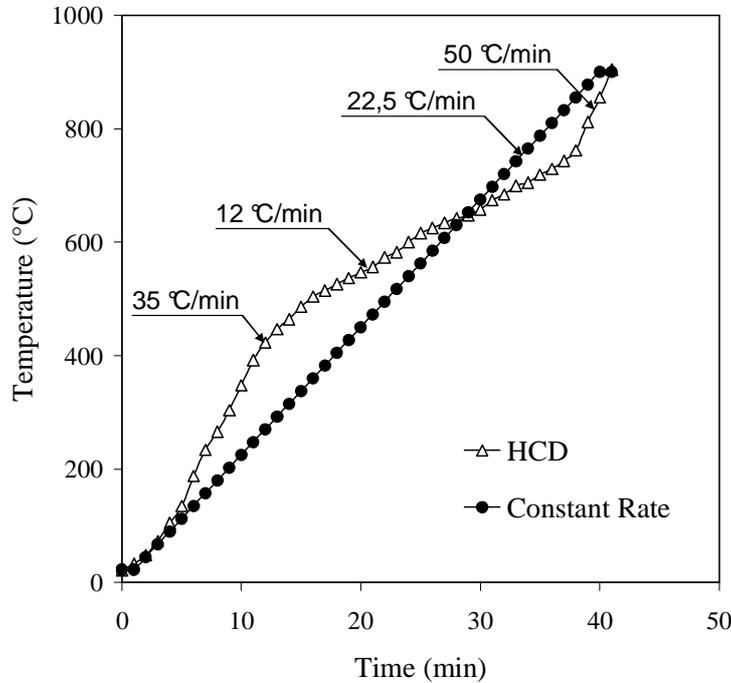
Figure 3. Heating curve obtained to reach the specified annealing temperature for the studied condition.
