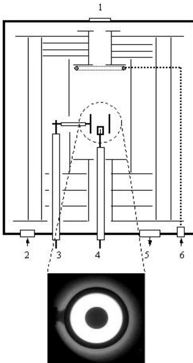
Figure 1. Schematic representation of the discharge chamber and an *in situ* photography of the hollow cathode discharge (1 = view window; 2 = outlet to manometer; 3 = external electrode; 4 = central electrode; 5 = outlet to vacuum pump; and 6 = gaseous mixture inlet).
