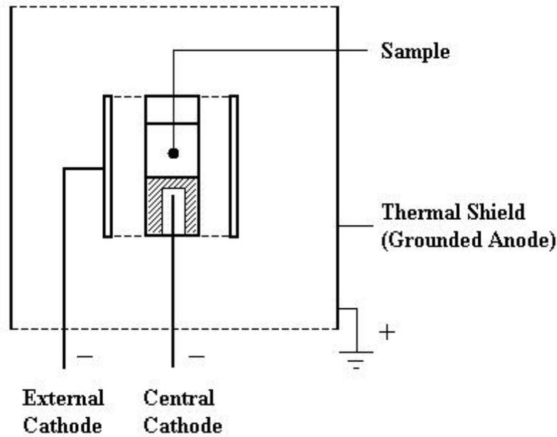
Figure 2. Schematic representation of the hollow cathode discharge configuration.
