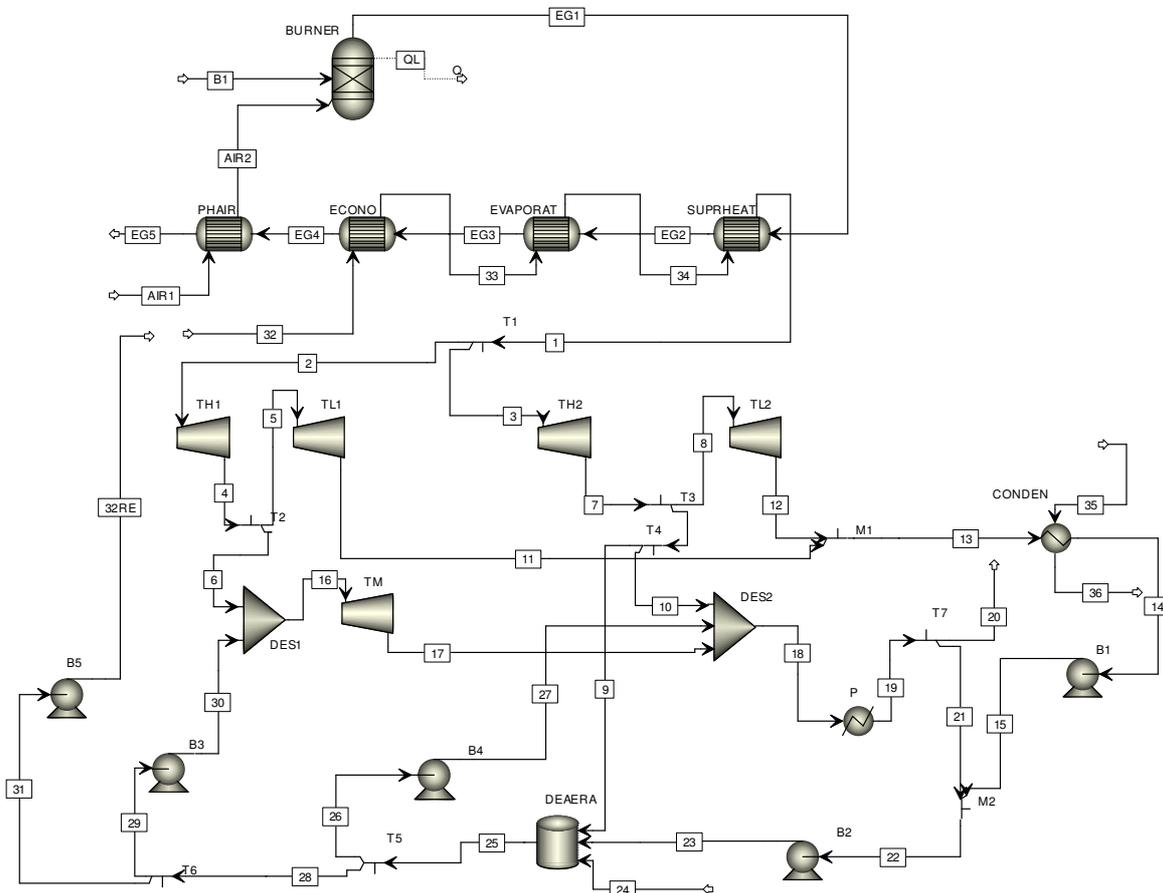
Figure 3. Scheme of the cogeneration system in ASPEN PLUS
