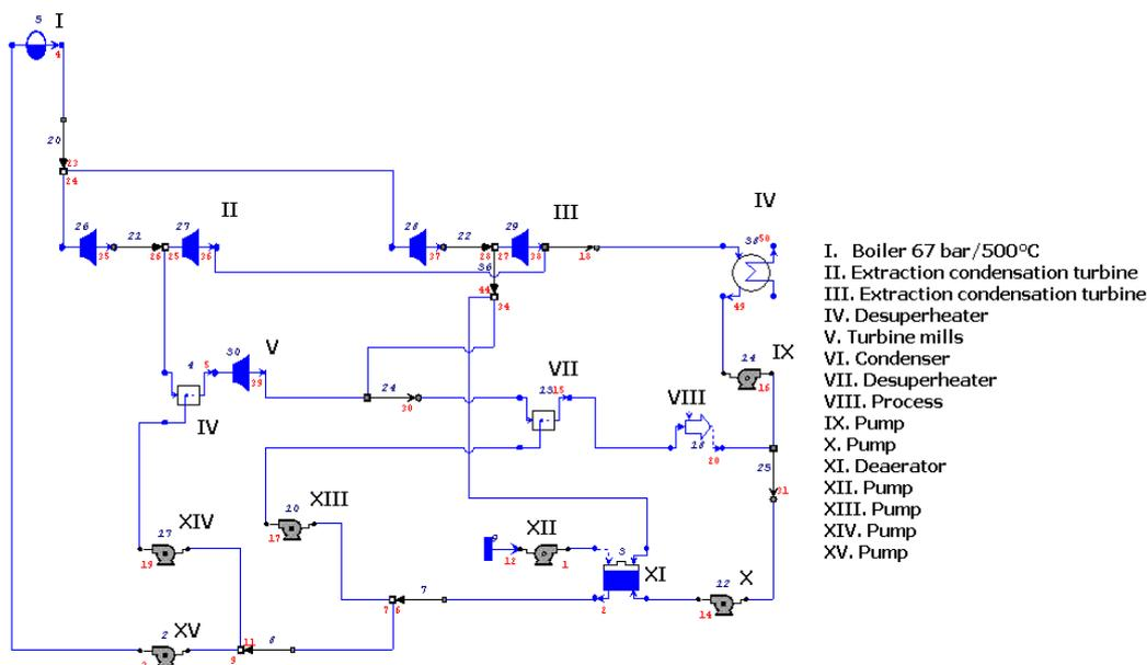
Figure 1. Diagram of the cogeneration system studied – Scheme of THERMOFLEX.
