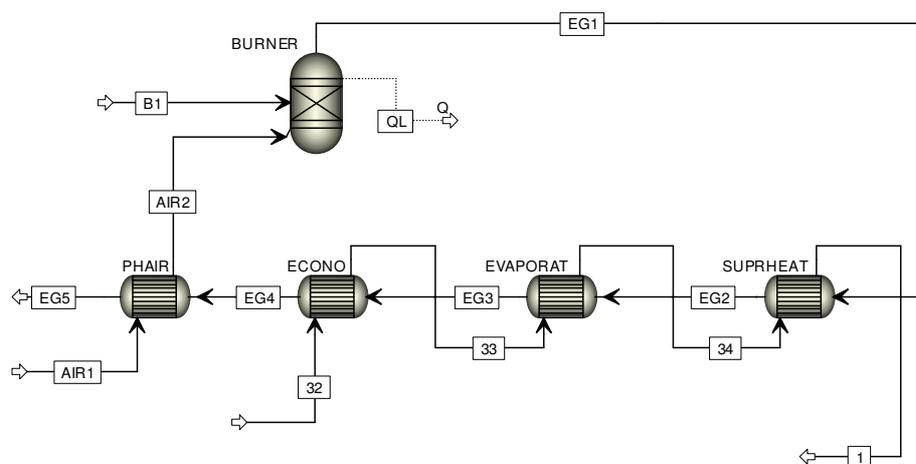
Figure 2. Scheme of the steam boiler in ASPEN PLUS
