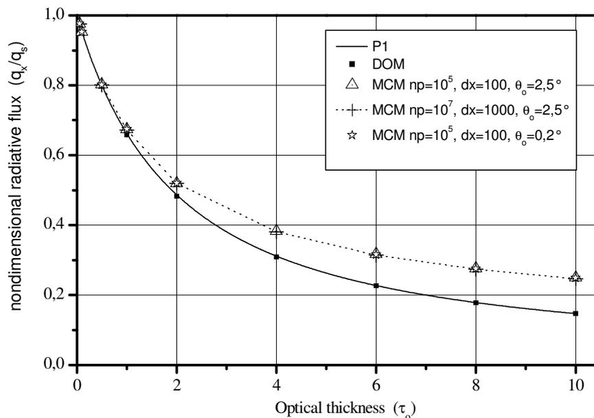
Figure 2. Comparison between DOM and MCM to a nondimensional radiative heat flux in a purely scattering layer with a normal collimated irradiation and isotropic scatter.
