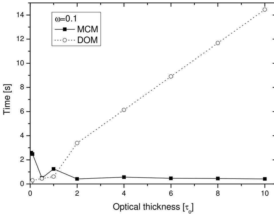
Figure 7. Computational time to MCM and DOM to albedo,  $\omega = 0.1$ .
