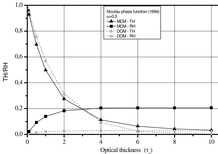
Figure 4. Hemispherical transmittance and reflectance to MCM and DOM to a unitary albedo,  $\omega=0.5$ , anisotropically scattering and Nicolau phase function.
