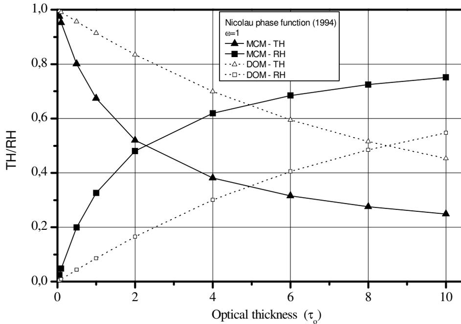
Figure 3. Hemispherical transmittance and reflectance to MCM and DOM to an unitary albedo,  $\omega=1.0$ , anisotropically scattering and Nicolau phase function.
