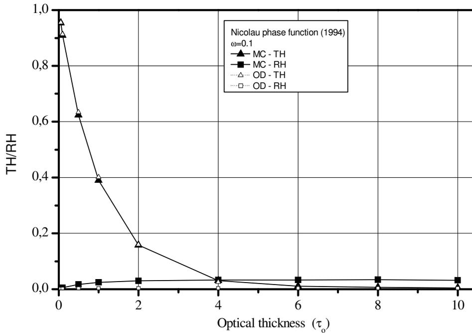
Figure 5. Hemispherical transmittance and reflectance to MCM and DOM to an unitary albedo,  $\omega=0.1$ , anisotropically scattering and Nicolau phase function.
