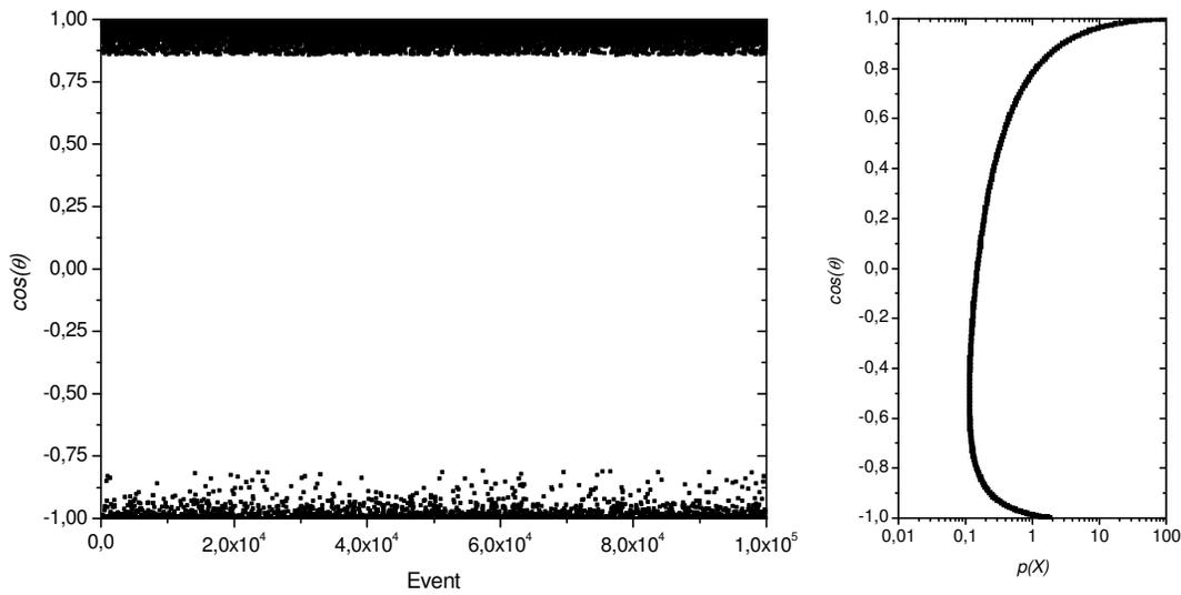
Figure 1. Anisotropic phase function randomly generated to 100,000 statistical realizations.  $g_1 = 0.86$ ;  $g_2 = 0.8$ ;  $f_1 = 0.96$ ;  $f_2 = 0.96$ .
