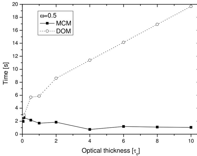
Figure 6. Computational time to MCM and DOM to albedo  $\omega = 0.5$ .
