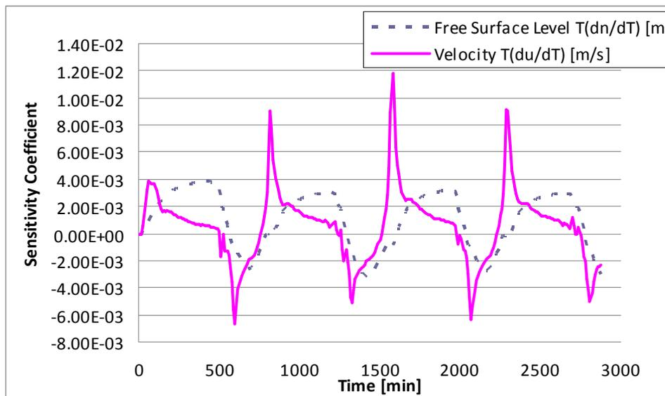
Figure 8 - Sensitivity coefficient for estimating the turbulent viscosity considering measurements taken at Station 2.
