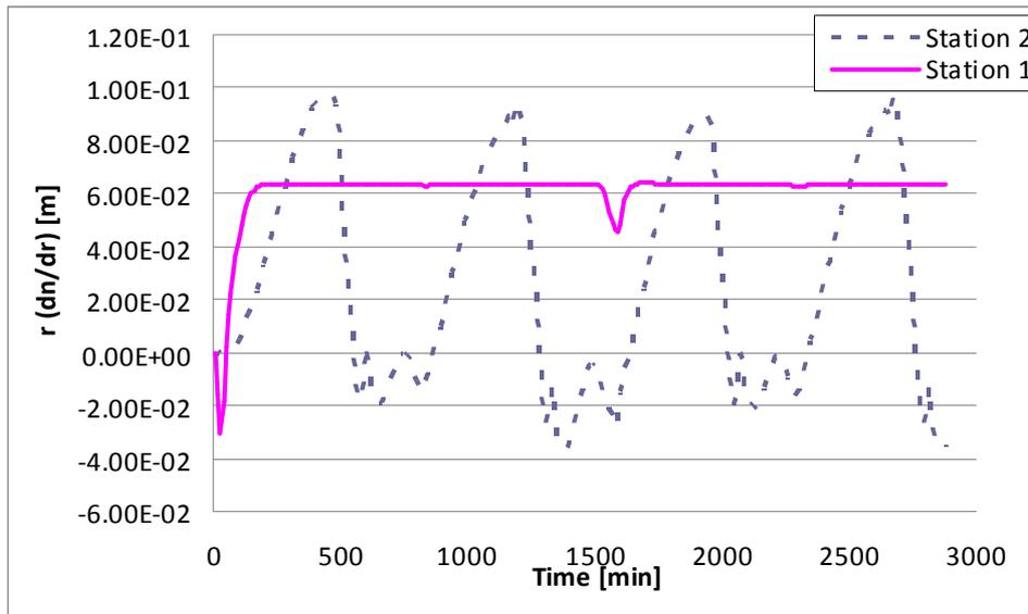
Figure 7 - Sensitivity coefficients for the estimation of the roughness height using free surface level measurements.
