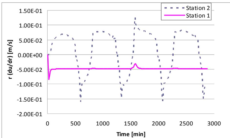
Figure 6 - Sensitivity coefficients for the estimation of the roughness height using velocity measurements.
