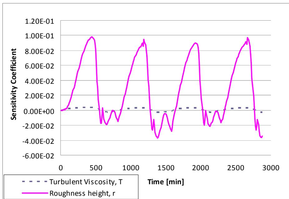
Figure 9 - Sensitivity coefficients considering measurements of free surface level taken at Station 2.
