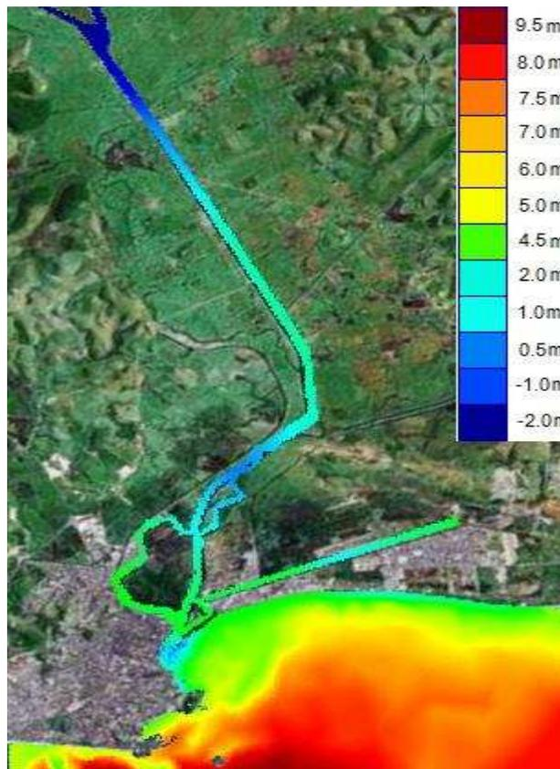
Figure 2 - Simulated domain and model bathymetry used.
