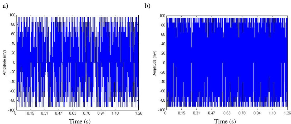
Figure 5 - Vibration signal in 1,26 seconds of drill 1: a) Tool in the state 1; b) Tool in the state 3.
