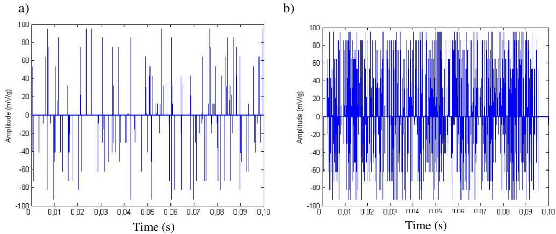
Figure 6 - Vibration signal in 0,1 seconds of drill 1: a) Tool in the state 1; b) Tool in the state 3.
