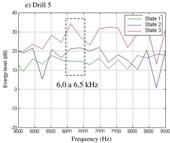
Figure 9. Spectrums in frequencies range from 4,5 to 9,0 kHz.
