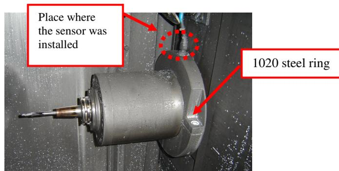
Figure 2. Vibration sensor installed.
