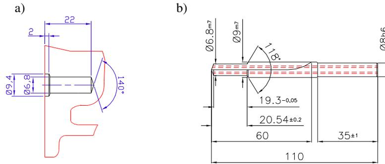
Figure 1. a) Hole characteristics b) Drill characteristics.
