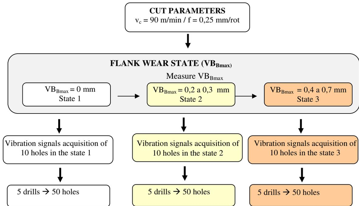
Figure 4. Acquisition signals methodology.
