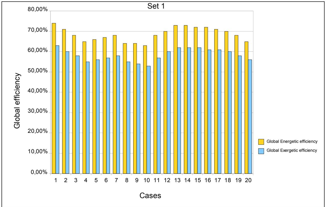
Figure 2- Efficiencies for set 1. [Efficiency is defined by the ratio between the delivered energy (mechanical plus steam for the process) and the energy of the fuel]
