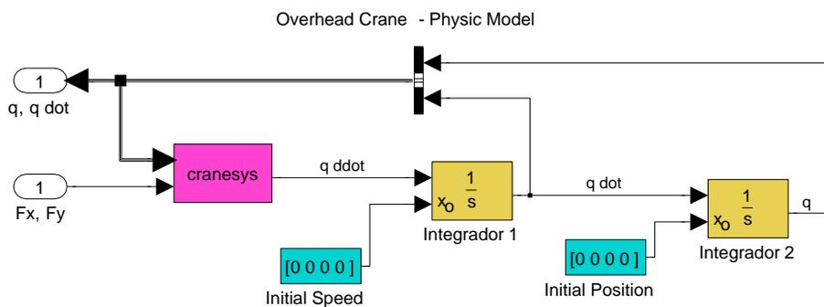
Figure 2: Physic model simulation diagram
