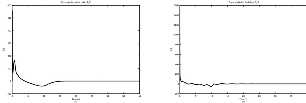
Figure 5: Simulation Results – forces applied by the actuator to (a) the trolley and (b) the bridge
