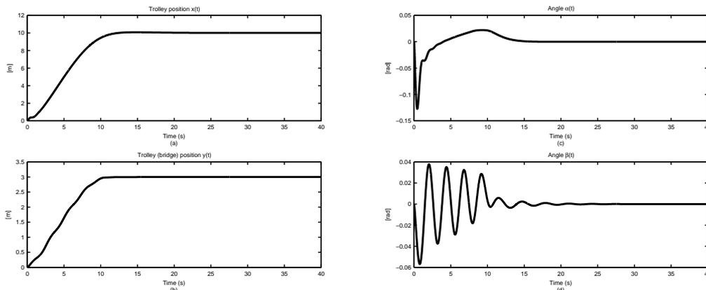
Figure 4: Simulation Results – positions  $x$  and  $y$ , and angles  $(\alpha$  and  $\beta)$
