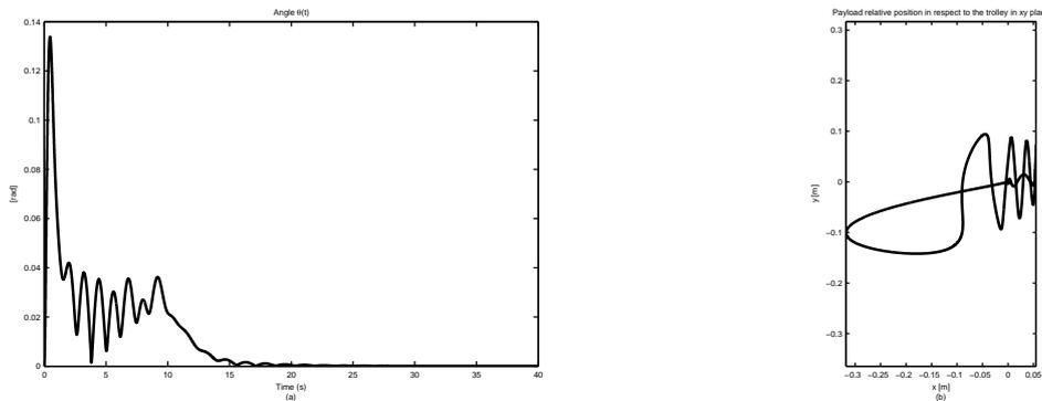
Figure 6: Simulation Results – (a) angles  $\theta$  and (b) payload relative position
