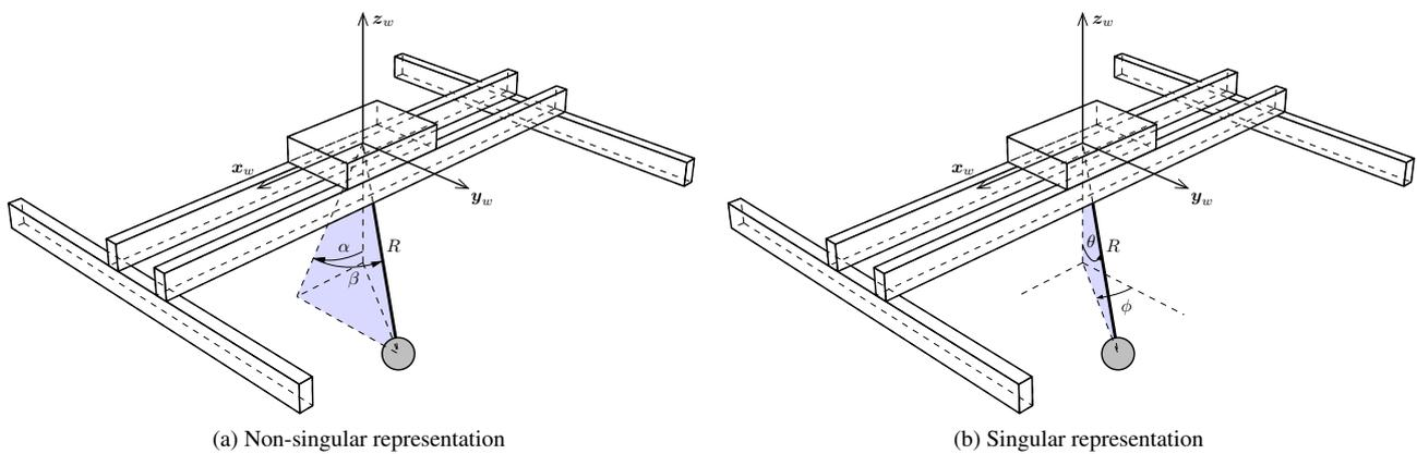
Figure 1: Schematic representation of an overhead crane
