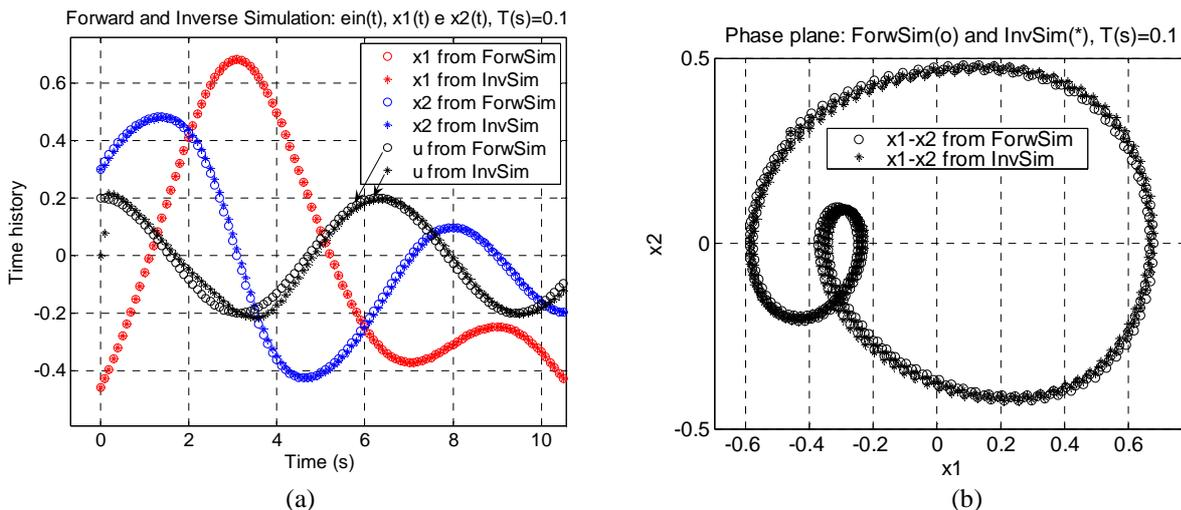
Figure 11. Results from Inverse Simulation for attractor A4,  $T = 100\text{ms}$ : (a) time histories and (b) Phase plane comparison
