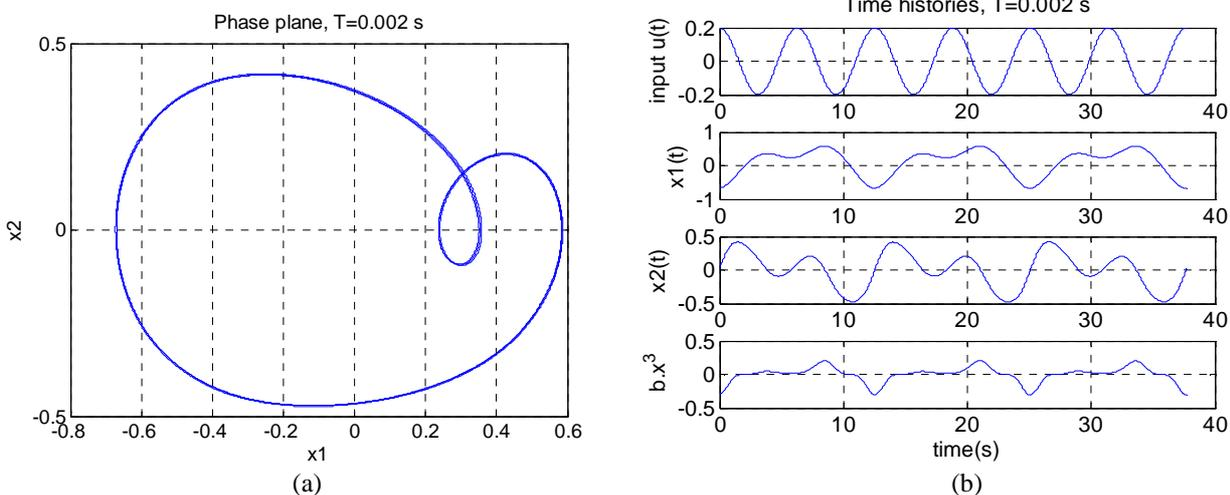
Figure 6. Forward simulation Duffing Equation, Attractor A3 (a) phase plane and (b)  $u(t)$ ,  $x_1$ ,  $x_2$  and  $x^3$  time histories
