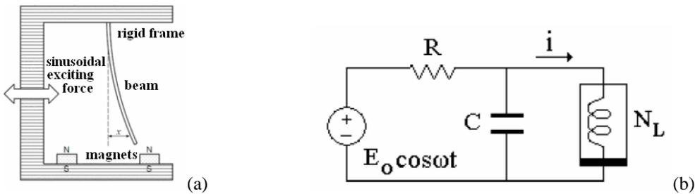
Figure 1. (a) Mechanical and (b) Electrical nonlinear oscillator
