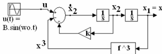
Figure 3. Duffing Equation Forward Simulation
