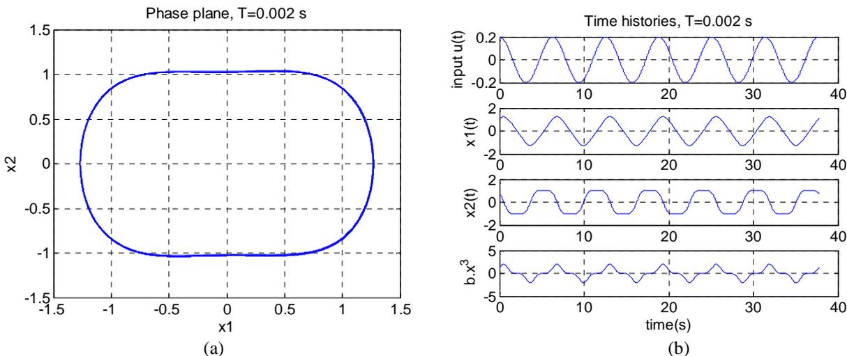
Figure 5. Forward simulation to Duffing Equation, Attractor A2 (a) phase plane
