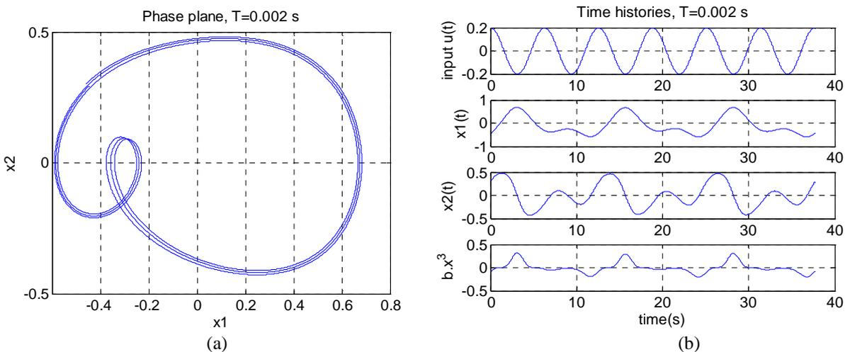
Figure 7. Forward simulation to Duffing Equation, Attractor A4 (a) phase plane
