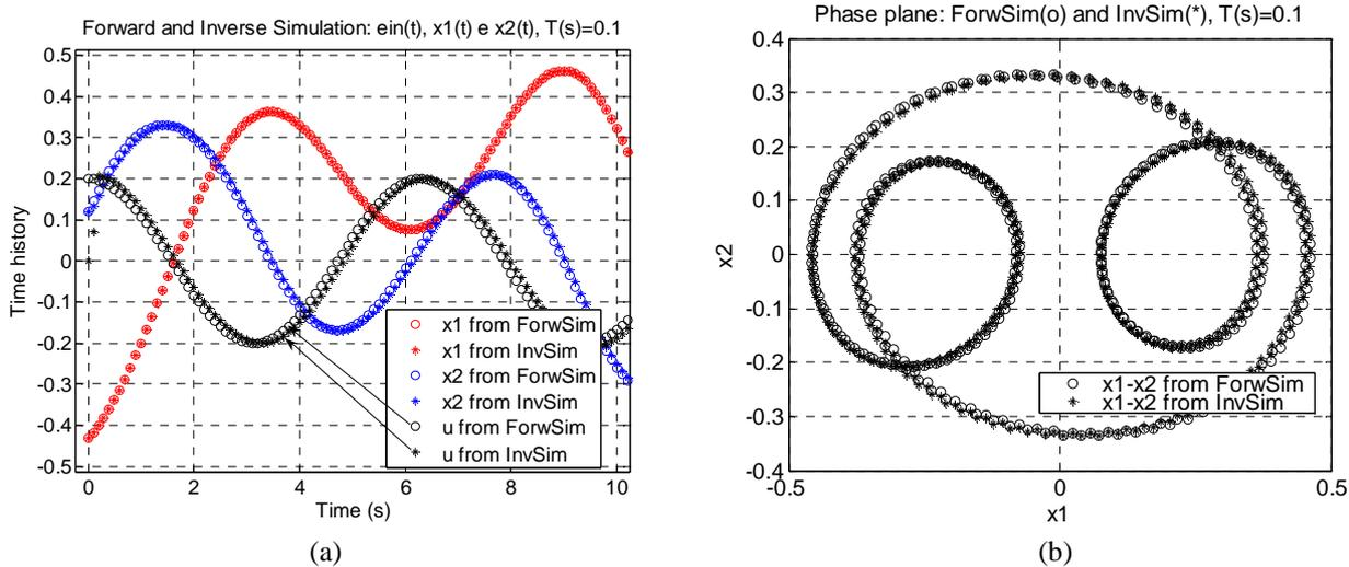
Figure 9. Results from Inverse Simulation, attractor A5,  $T = 100\text{ms}$  (a) Time histories (b) Phase plane comparison
