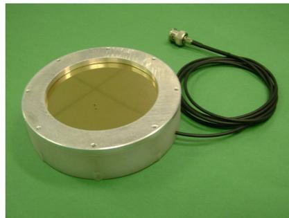
Figure 4. Large-aperture PVDF receiver.
