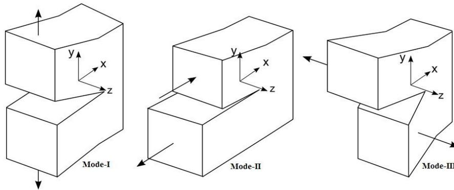
Figure 1. Crack opening modes.
