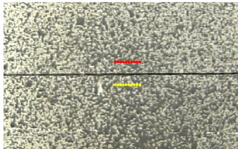
Figure 3. Control points positioned to determine the COD.
