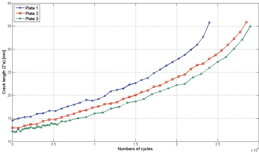
Figure 6. Curves of crack length by number of cycles to the three plates tested.
