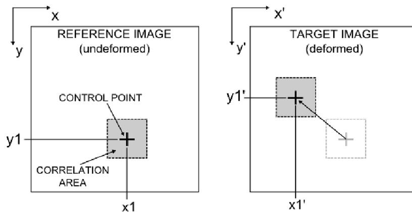
Figure 2. Correlation area around the control point and displacement of the control point.
