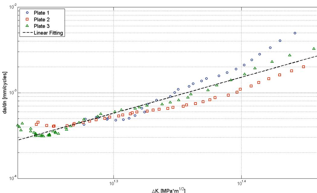
Figure 7. Curves  $\Delta K_I \times da/dn$  of three plates tested.
