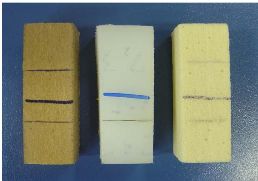
Figure 6: Marking tests made on the studied materials: MDF, Nylon and PU, respectively. Marks from top to bottom: pen, marker and pencil.
