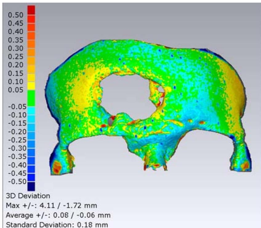
Figure 4: Color graphic presenting the precision of the PU biomodel.
