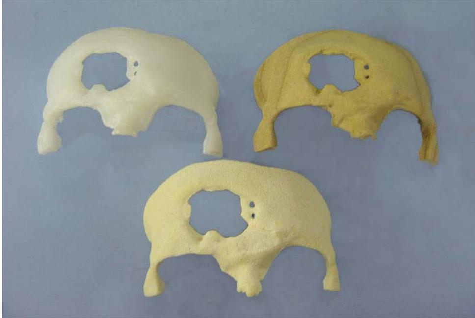
Figure 2: Biomodels manufactured via CNC milling.
