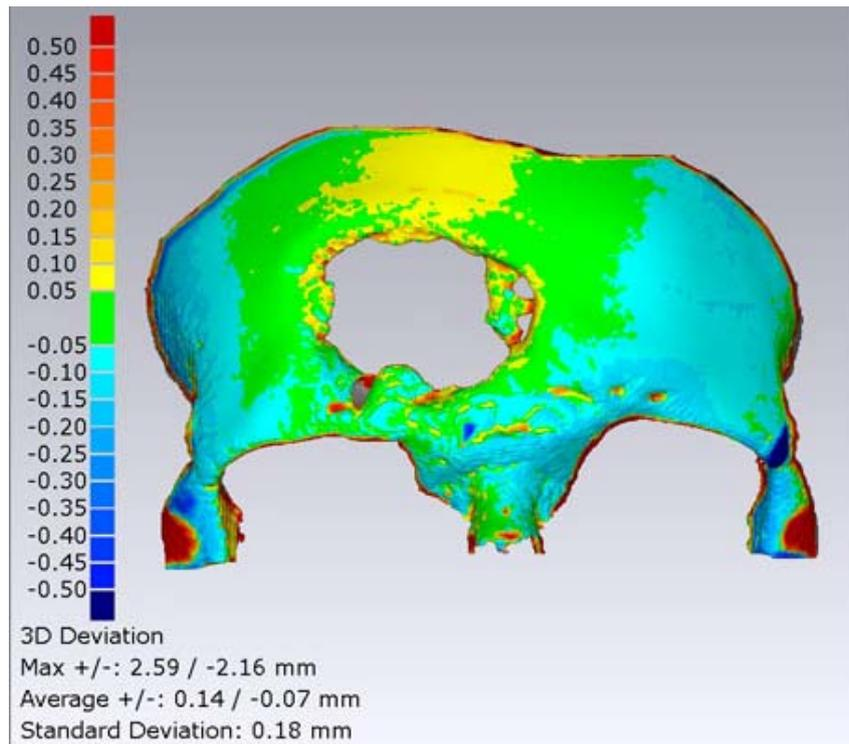
Figure 5: Color graphic presenting the precision of the Nylon biomodel.
