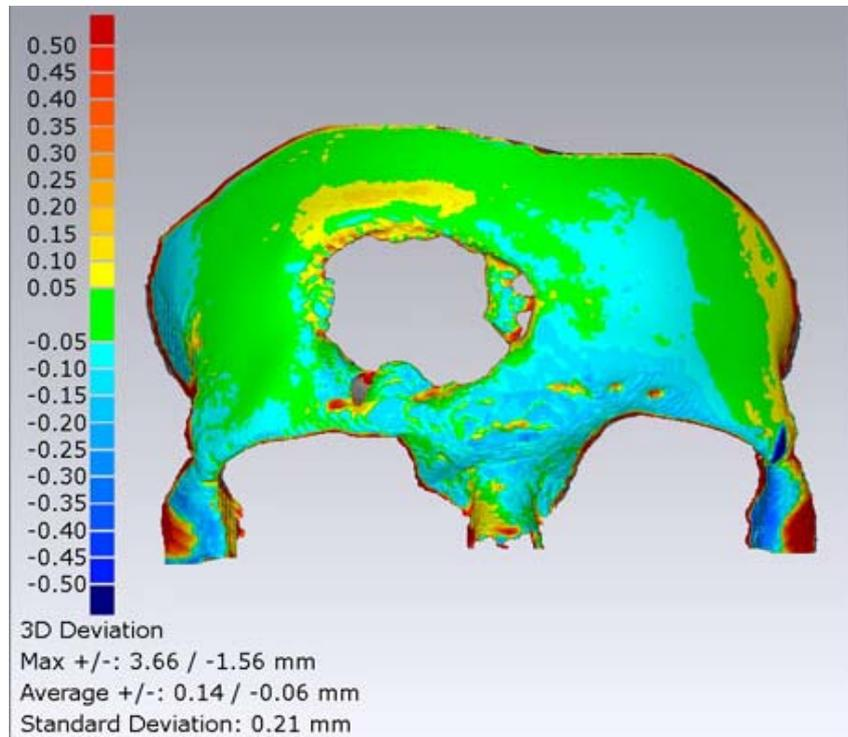
Figure 3: Color graphic presenting the precision of the MDF biomodel.
