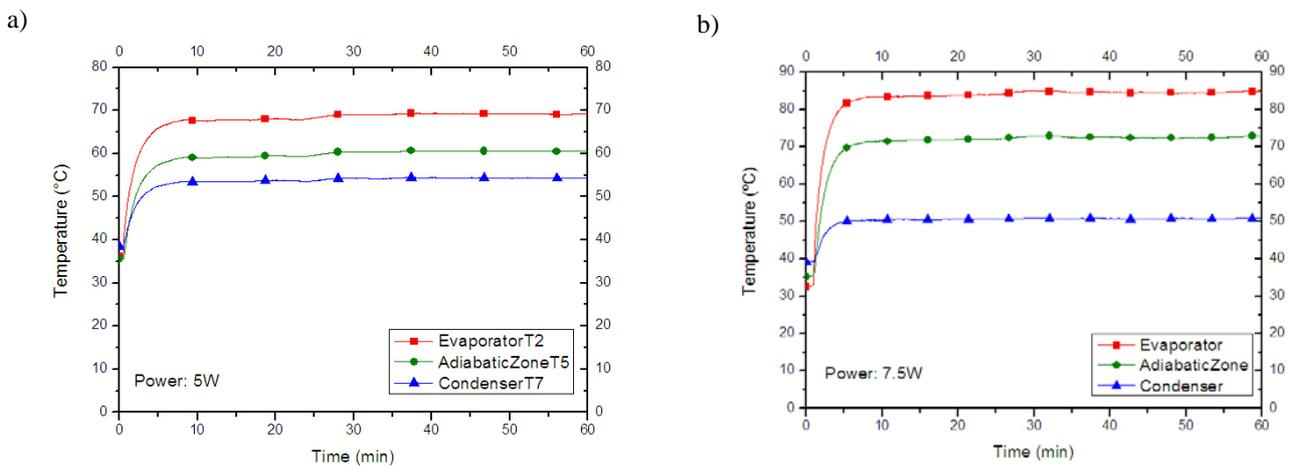
Figure 12. Temperature versus time in second heat pipe design: a) power applied 5W and b) 7.5W.
