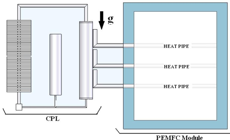
Figure 9. Integrated cooling system with heat pipe assisted by thermosyphon.
