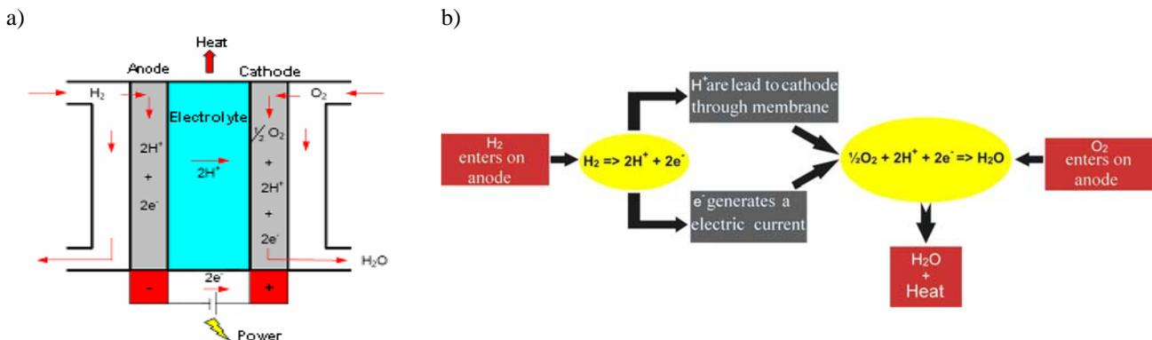
Figure 1.a) Operation scheme of PEMFC. b) Flowchart of reactants and products in a PEMFC.
