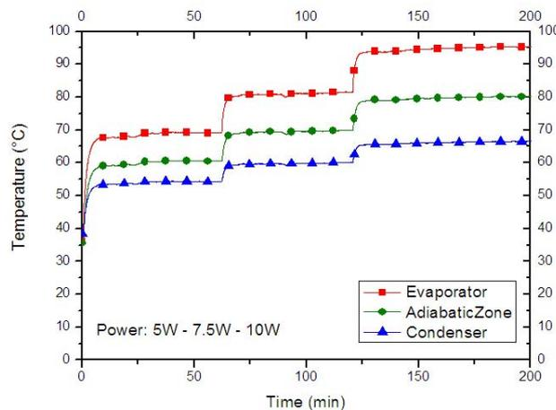
Figure 13. Power in different and successive applications in conventional heat pipe.
