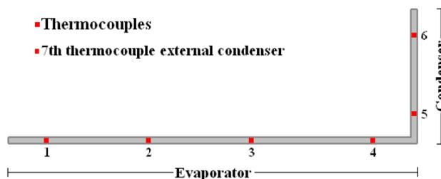
Figure 11. Thermocouples position along the second heat pipe design
