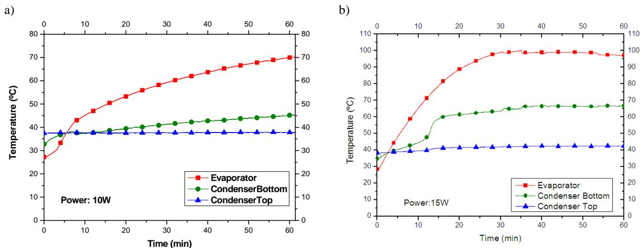
Figure 14. Temperature versus time in heat pipe assisted by thermosyphon: a) power applied 10W and b) 15W.
