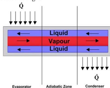
Figure 2. A heat pipe scheme showing the evaporator, adiabatic zone and condenser area.
