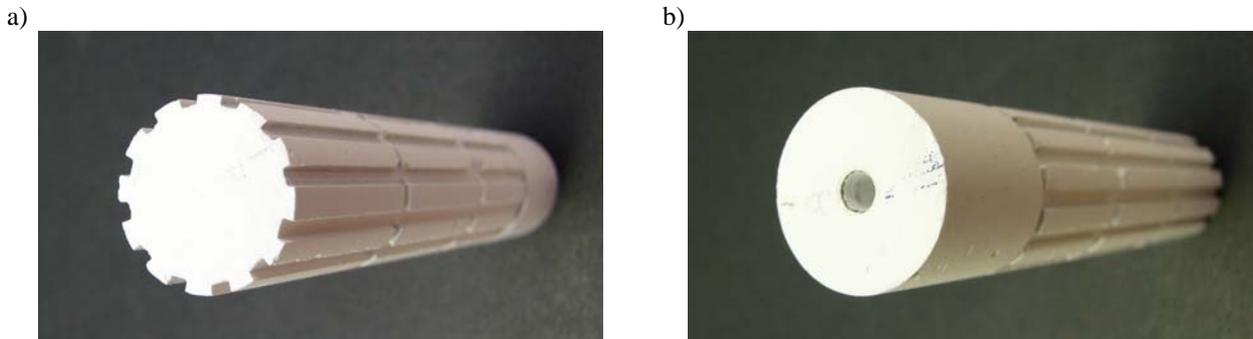
Figure 6. Porous ceramic structure of CPL a) vapour channels and b) liquid channel.
