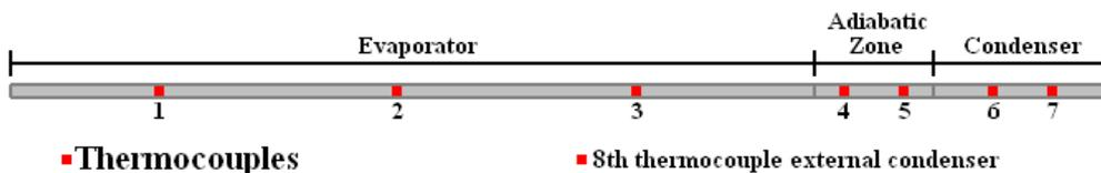
Figure 10. Thermocouples position along the first heat pipe design.
