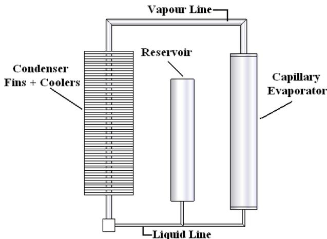
Figure 7. Scheme of CPL (in construction).
