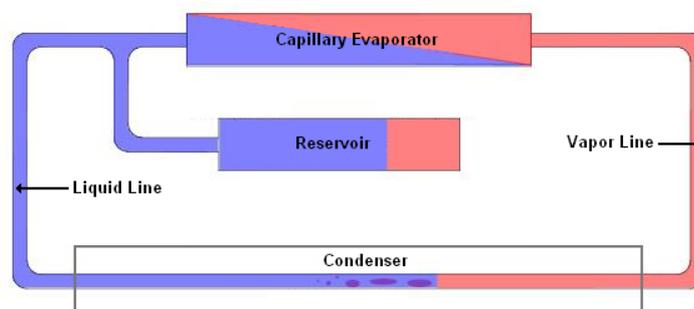
Figure 5. Capillary Pumped Loop (CPL).
