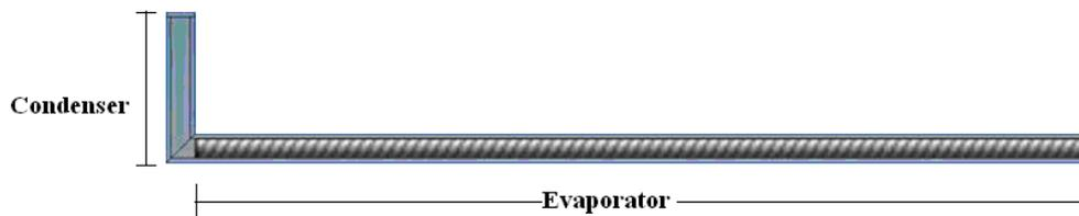
Figure 4. Heat pipe assisted by thermosyphon.
