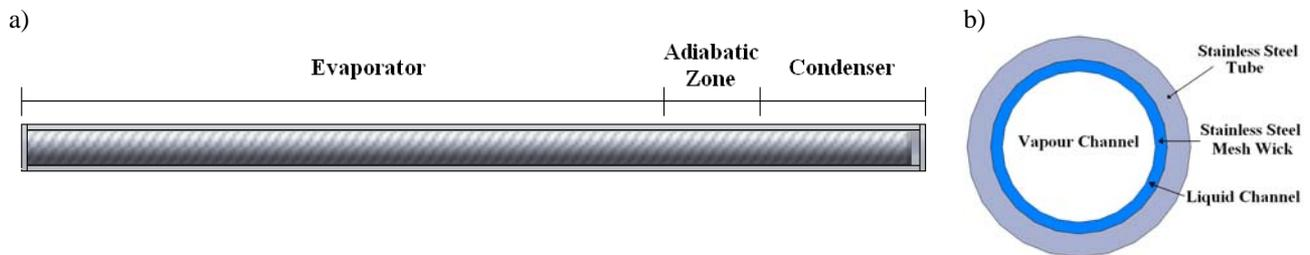
Figure 3. a) Conventional heat pipe in lateral view. b) Heat pipe section view.
