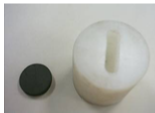
Figure 7. Picture of a sabot and a rubber specimen
