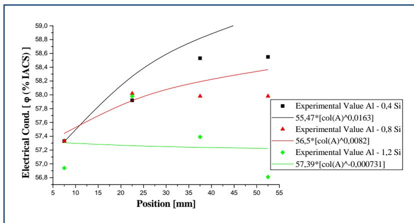
Figure 12. Electrical conductivity in relation of the position the wire 3.98 mm diameter
