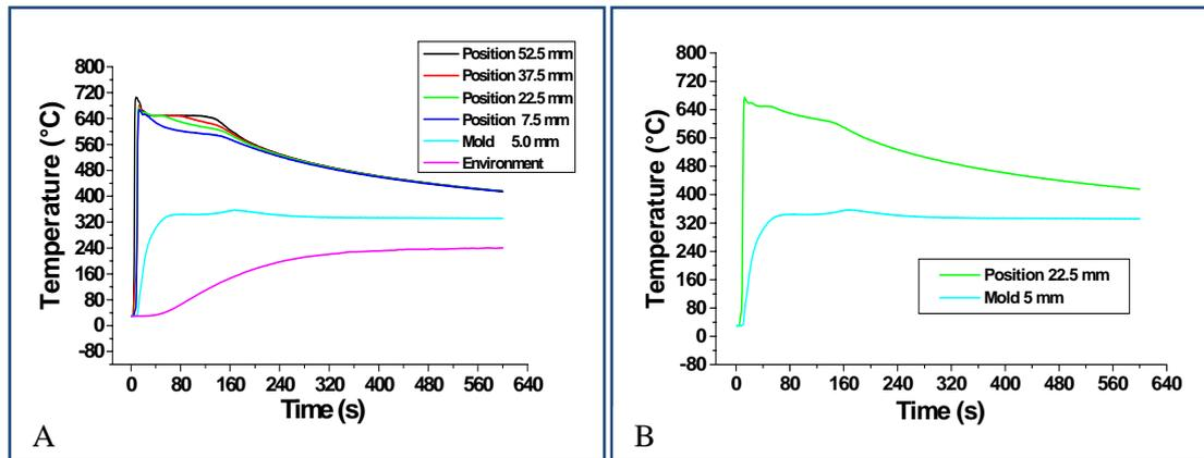
Figure 5. [A] Experimental Thermal Profile obtained of pouring for Al-0.6%Si-0.7%Mg alloy, [B] Thermal Profile of the metal in 22.5 mm position associated to mold profile in 5 mm distance
