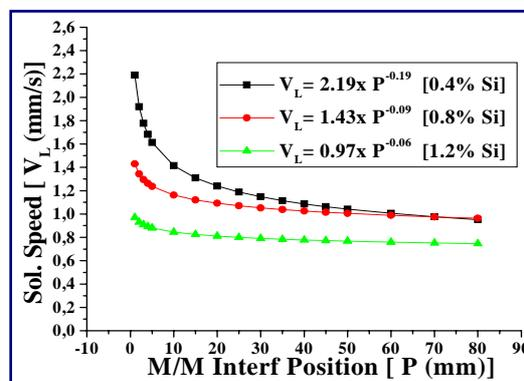
Figure 7. Curves describes the speed variation of liquidus isotherm ( $V_L$ ) with M/M interface distance in function of Si evolution
