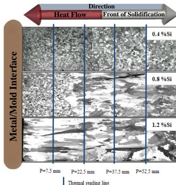
Figure 9. Macrograph of the modified alloys with Si contents proposed
