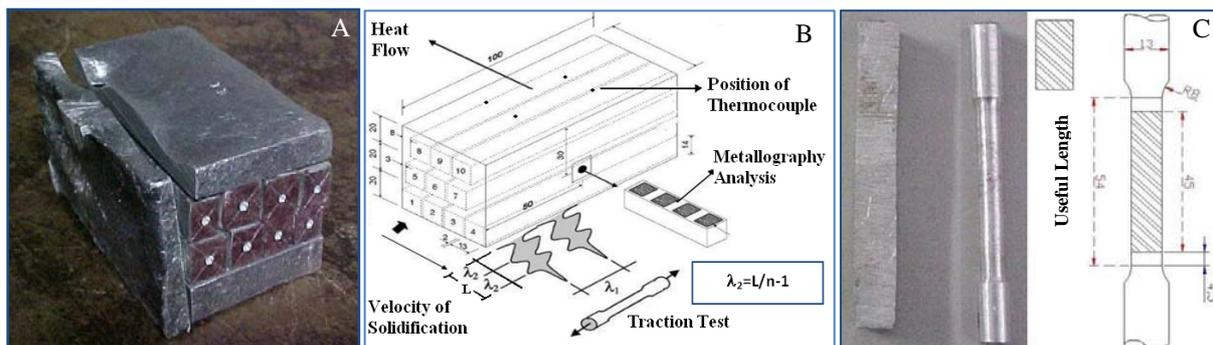
Figure 3. Disposal of the Test Specimens removal: On [A], Photo showing the cut ingot obtained satisfying the provisions on [B], which shows the direction of dendritic evolution in relation to tension specimen collection; On [C], Photo illustrating the bar of square cross section after cutting the ingot and the fabricated test specimen with test specimen dimensions according to ASTM-E8M norm.
