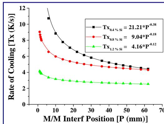
Figure 8. Correlation between Rate of Cooling and Position in relation to M/M Interface and Solute content of the alloys: variation in Si content
