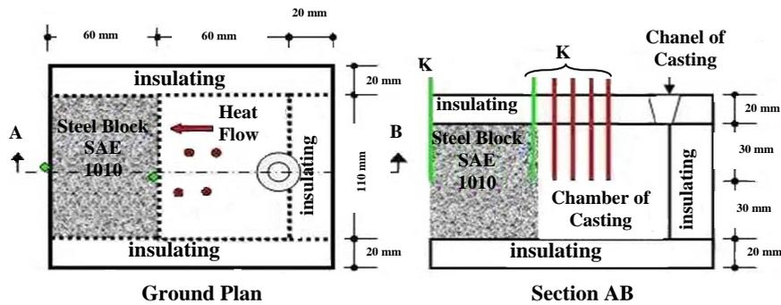
Figure 1. Top and side view of pouring chamber with thermocouples installed in previously chosen positions [Mattos, 2005]
