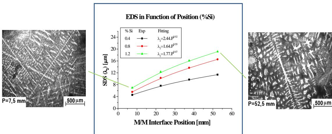
Figure 11. SDS in function of position and micrographic photo
