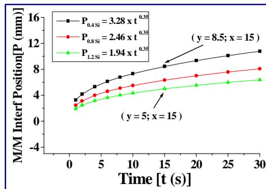
Figure 6. Evolution of Liquidus Isotherm Profiles of the studied alloys, variation on Si content
