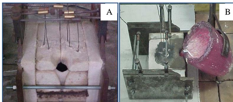
Figure 2. [A] Pouring Chamber and the Thermocouple disposal and [B] Alloy Pouring on Chamber
