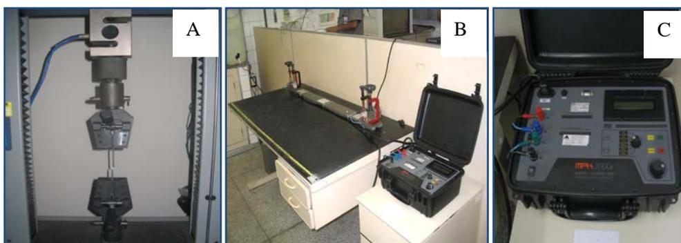
Figure 4. [A] Equipments for Mechanical [KRATOS] and [B;C] Electrical [Micro Ohmeter – Kelvin bridge, MEGABRÁS MPK-2000 model] Characterization
