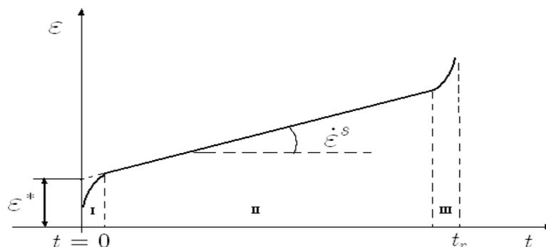
Figure 6: Typical experimental creep curve
