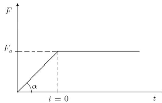
Figure 4: Typical loading history in a long term creep test
