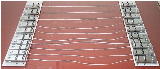
Fig. 2 A sample of HMPE creep specimens
