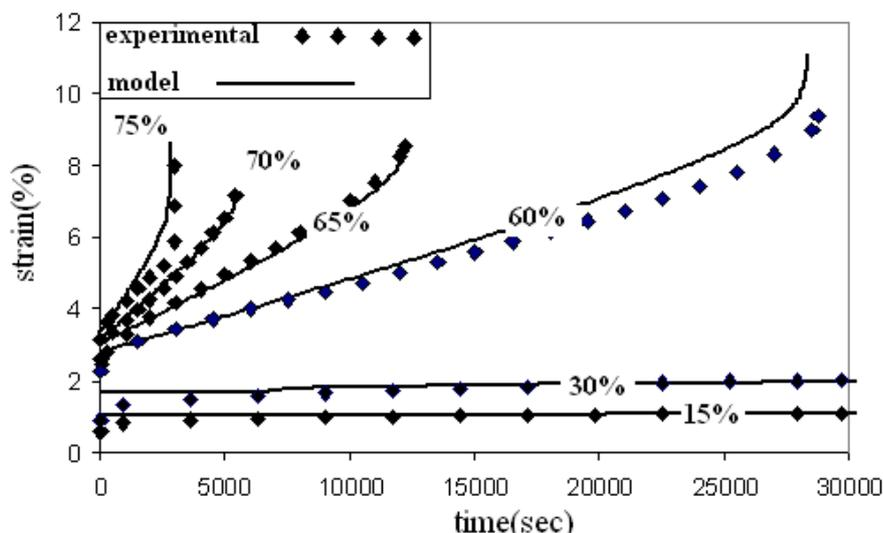
Figure 11: Creep curves at different load levels. Comparison with experimental results.
