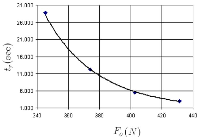
Figure 10: Creep lifetimes for different load levels. Comparison with experimental results.
