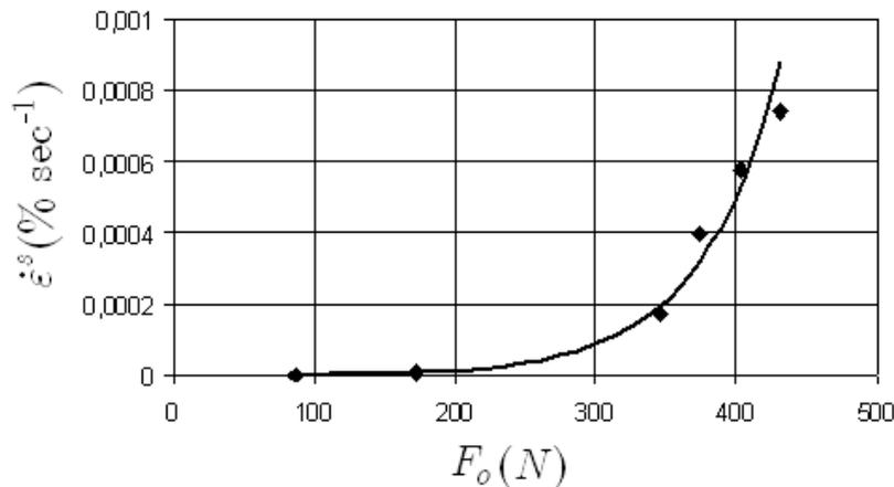
Figure 8: Secondary creep rate for different load levels. Comparison with experimental results.  $\alpha = 8,3$  N/sec
