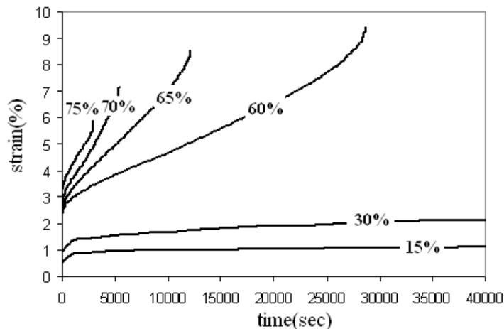
Figure 5: Experimental creep curves at different load levels.
