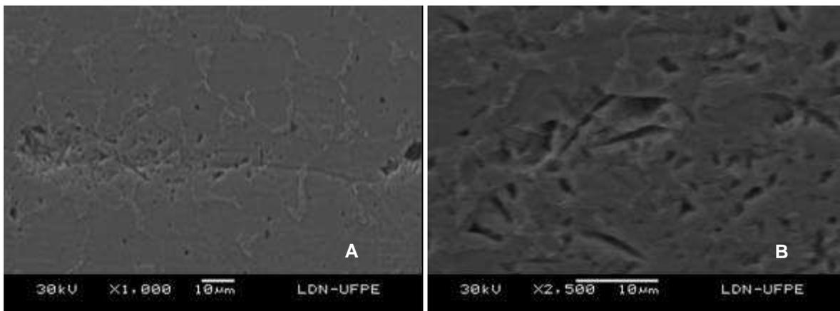
Figure 3 - Micrographs of the root (A) and of the molten metal (B) of the welded joint with the mixture (Ar 75% / 25% CO<sub>2</sub>) as shielding gas.
