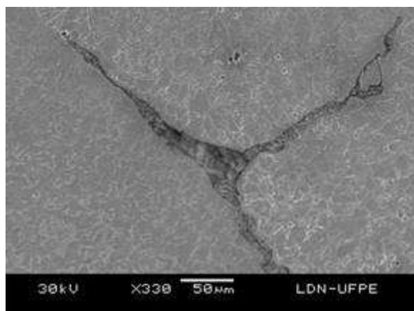
Figure 1 - Micrography of the root of the welded joint with the Ar as shielding gas.
