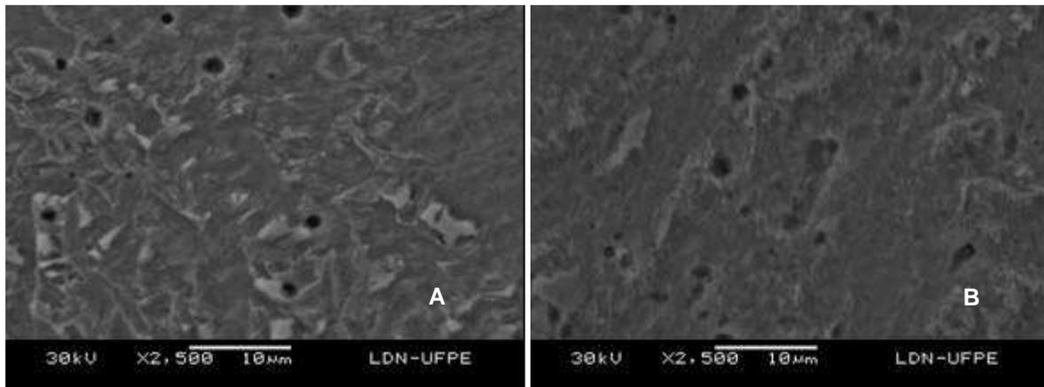
Figure 2 - Micrographs of the molten metals of the welded joints with the Ar (A) and with the CO<sub>2</sub> (B) as shielding gases.
