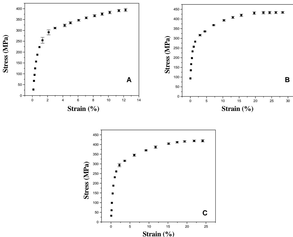
Figure 4 – Curves Stress ( $\sigma$ ) X Strain (%) of the welded joints with the Ar (A), the mixture (B) and the CO<sub>2</sub> (C) as shielding gases.
