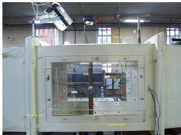
Figure 2. Test section of the wind tunnel.
