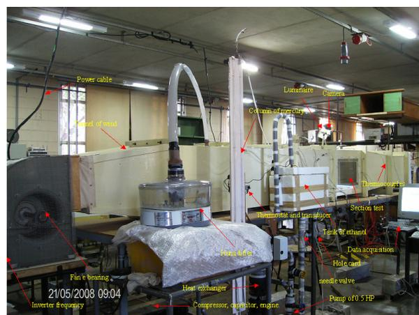
Figure 3. The tunnel and the experimental system.
