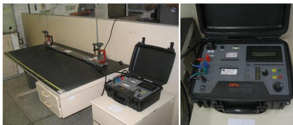
Figure 5. Photos of a component set of Kelvin bridge utilized.
