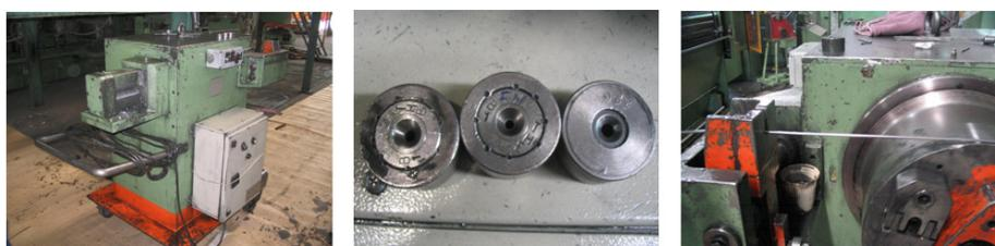
Figure 4. Drawing frame, diamond wire gage utilized ( $\varnothing=3.6\text{mm}$  3.18mm e 2.89mm) and the drawing moment.
