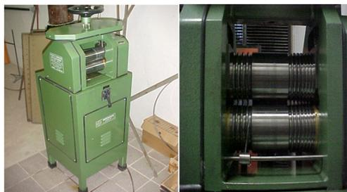
Figure 3. Electrical rolling mill utilized.
