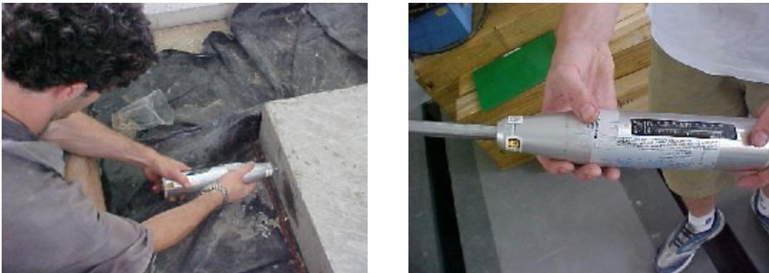
Figure 1. The Sclerometer Test
