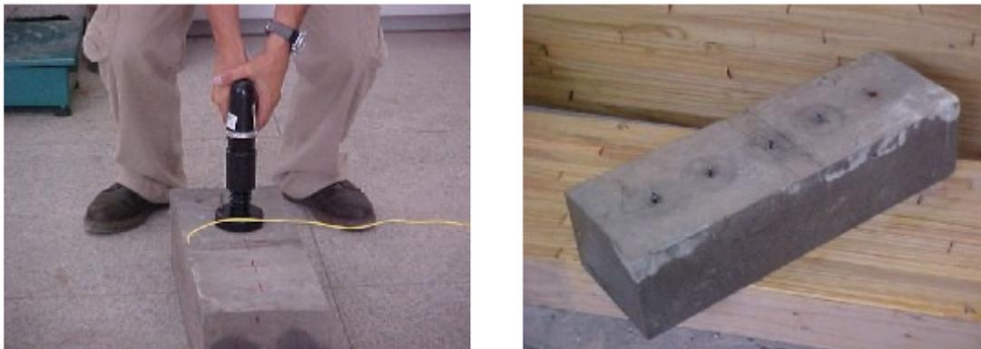
Figure 2. Pin Penetration Test
