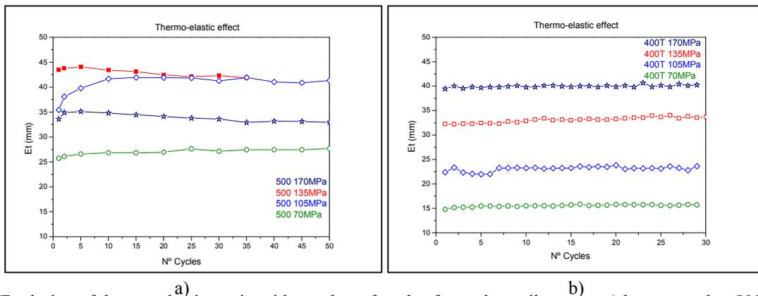
Figure 5. Evolution of thermo-elastic strain with number of cycles for each tensile stress. a) heat treated at 500T b) heat treated at 400T.
