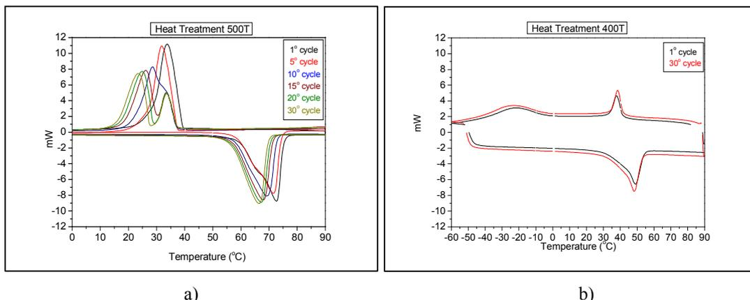
Figure 6. Calorimetric cycles for samples heat treated a) 500T b) 400T.
