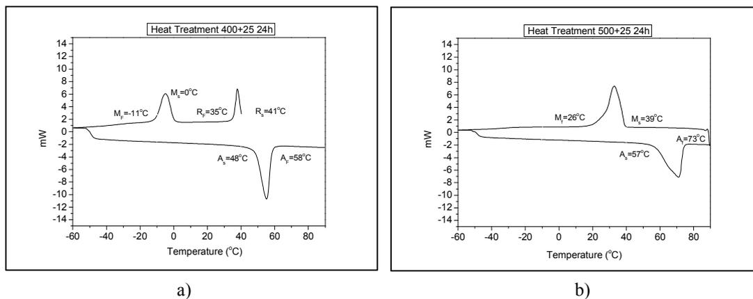
Figure 1. Calorimetric curves. a) Sample heat treated at 400°C for 24 hours and b) Sample heat treated at 500°C for 24 hours.
