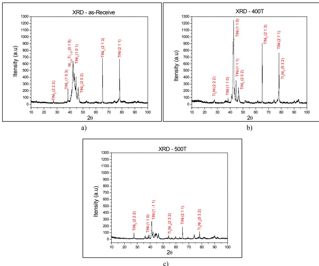
Figure 2. X-Ray diffraction results. a) as-receive sample b) heat treated at 400T and c) heat treated at 500T.
