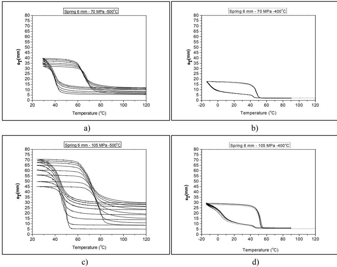
Figure 3. Strain-temperature curves obtained during consecutive training cycles under tensile stress: a) and b) 70 MPa, c) and d) 105 MPa, (1, 2, 5, 10, 20 and 30 cycles).
