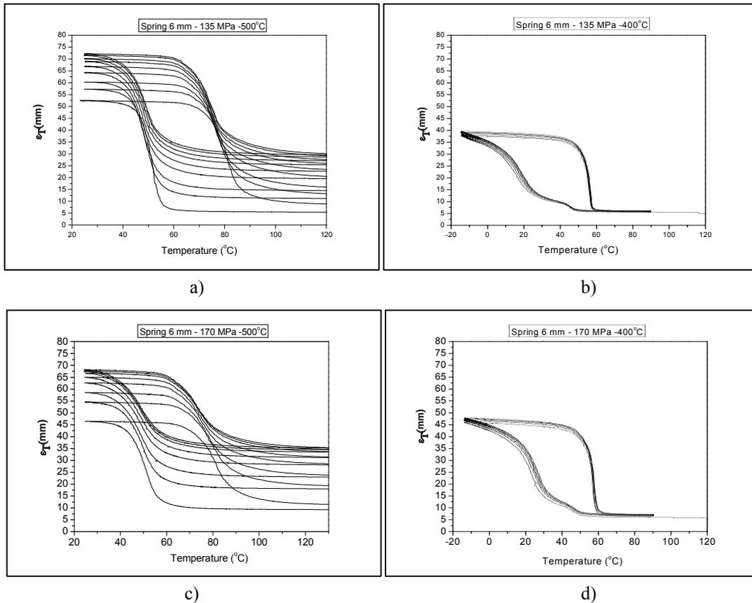
Figure 4. Strain-temperature curves obtained during consecutive training cycles under tensile stress: a) and b) 135 MPa, c) and d) 170 MPa, (1, 2, 5, 10, 20 and 30 cycles).
