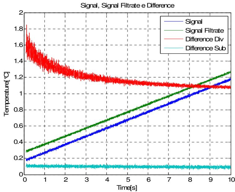
Figure 12. Signals that pass through the filter of 10Hz used in the output of the sensor of temperature, with the input signal, the filtered signal and the difference between these signals.
