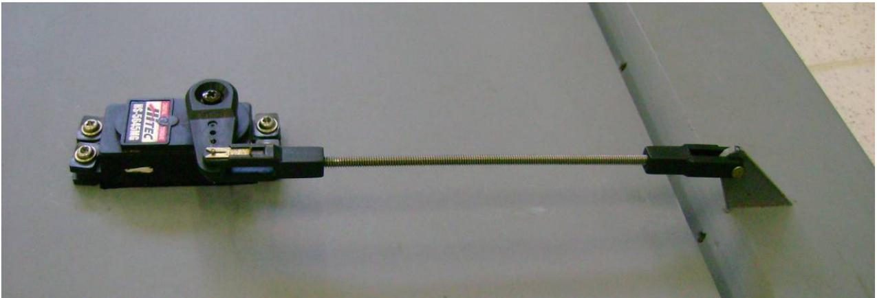
Figure 16. Servo modified at the surface of aerodynamic control.
