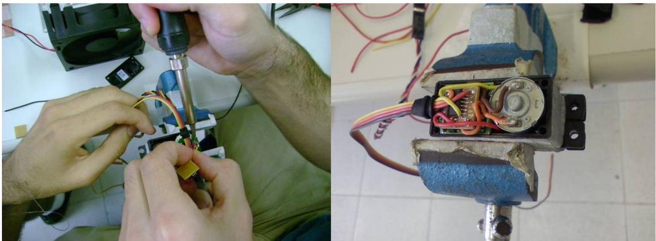
Figure 6. Left picture of the modification of the servo, the right shows the internal adapter already installed on the servo.
