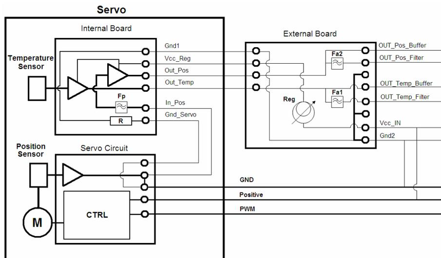
Figure 8. The block diagram of the modification of the servo actuator, with the inner board (internal circuit) and external adapter (external circuit).
