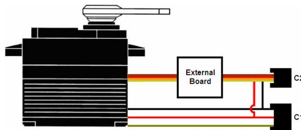
Figure 5. Illustration of the servo with the external adapter and connections after the modification
