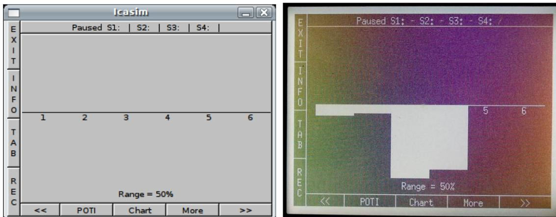
Figure 4: Panel of the bar graph from the PotiAMP (left layout, right photo).
