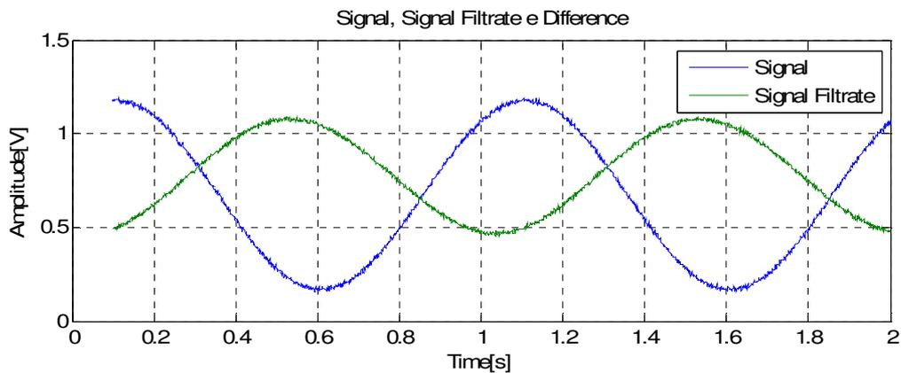
Figure 10. Shows the injected signal and filtered signal (test of the response of the filter).
