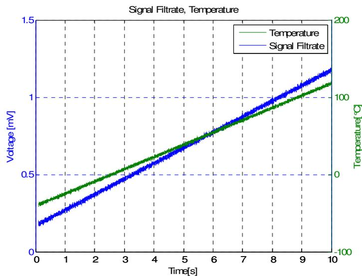
Figure 13. Showing the output signal (unfiltered) from the temperature sensor signal and the equivalent temperature in ° C
