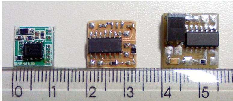
Figure 7. Versions of the inner board, left to right is in the versions (2.0, 1.1 and 1.0), the scale is in centimeters.
