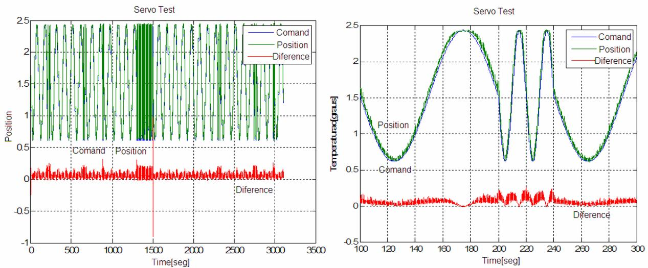
Figure 14. Sign of control, and position error (between control and position): a test of the left and right 3500 seconds in a zoom window of 5 minutes of test
