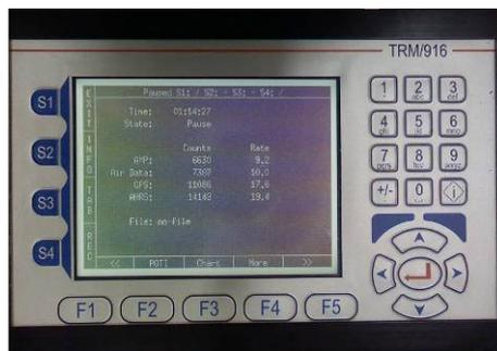
Figure 3. TRM/916 highlighting the buttons to control S1 to S4, the F1 and F4 and directional keypad on the right
