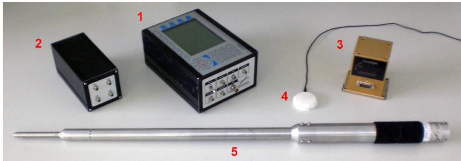
Figure 4. (1) TRM/916, (2) PotiAMP, (3) Crossbow AHRS400, (4) GPS antenna and (5) Anemometric probe.
