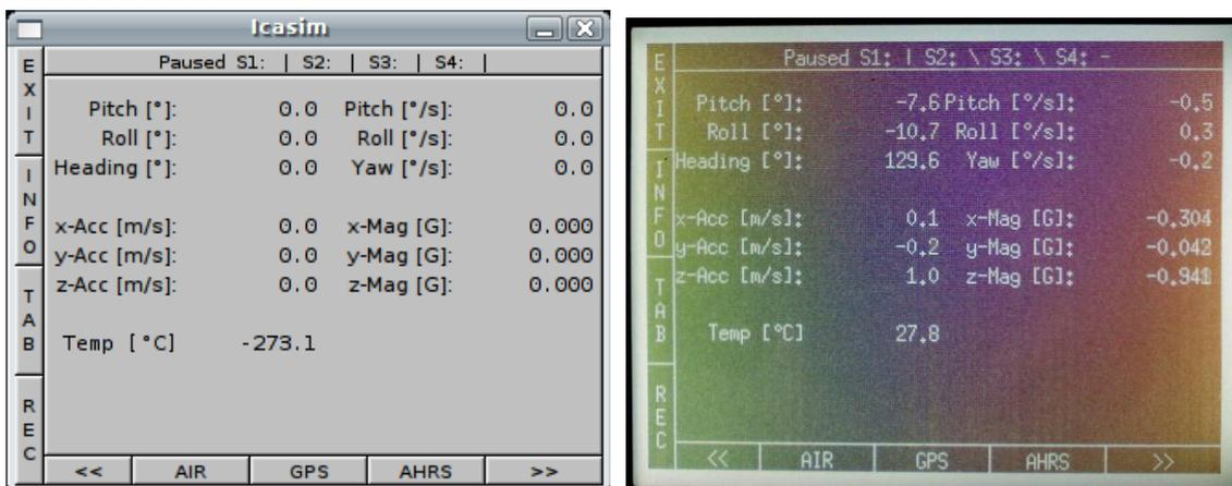
Figure 6. Scoreboard inertial unit (left layout, right photo). Which contains information from the inertial AHRS unit such as: Pitch, Pitch-rate, roll, roll-rate, Heading, Yaw, Acc x-, y-Acc, Acc-z, x-Mag, Mag-y, and z-Mag Temp.
