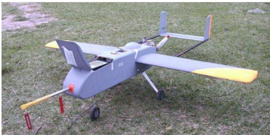
Figure 13. Vector-P after the changes where you can see the anemometer probe and TRM/916
