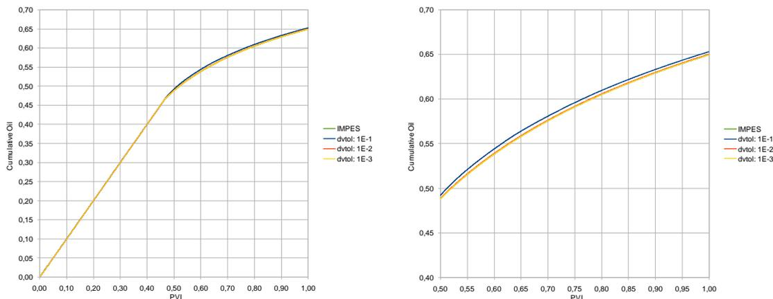
Figure 4. Cumulative oil for the ¼ homogeneous five-spot problem with the classical IMPES and with the MIMPES for DVTOL ranging from  $10^{-3}$  to  $10^{-1}$  (zoom on the right of the figure).
