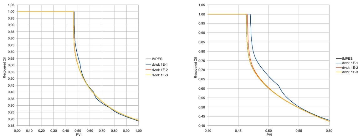
Figure 3. Recovered oil for the  $\frac{1}{4}$  homogeneous five-spot problem with the classical IMPES and with the MIMPES for DVTOL ranging from  $10^{-3}$  to  $10^{-1}$  (zoom on the right of the figure).
