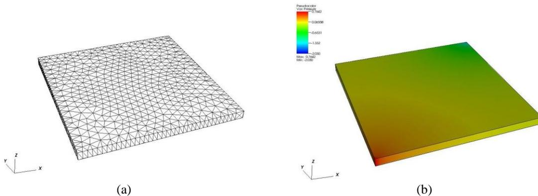
Figure 1.  $\frac{1}{4}$  homogeneous five-spot: a) Computational Mesh with 1236 nodes and 3892 tetrahedral elements; b) Pressure Field at  $t=1.0$  PVI obtained with the classical IMPES method.
