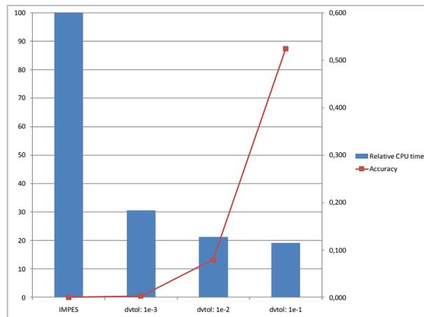
Figure 5. CPU time and relative difference of the cumulative oil between the classical IMPES and MIMPES for DVTOL ranging from  $10^{-3}$  to  $10^{-1}$ .
