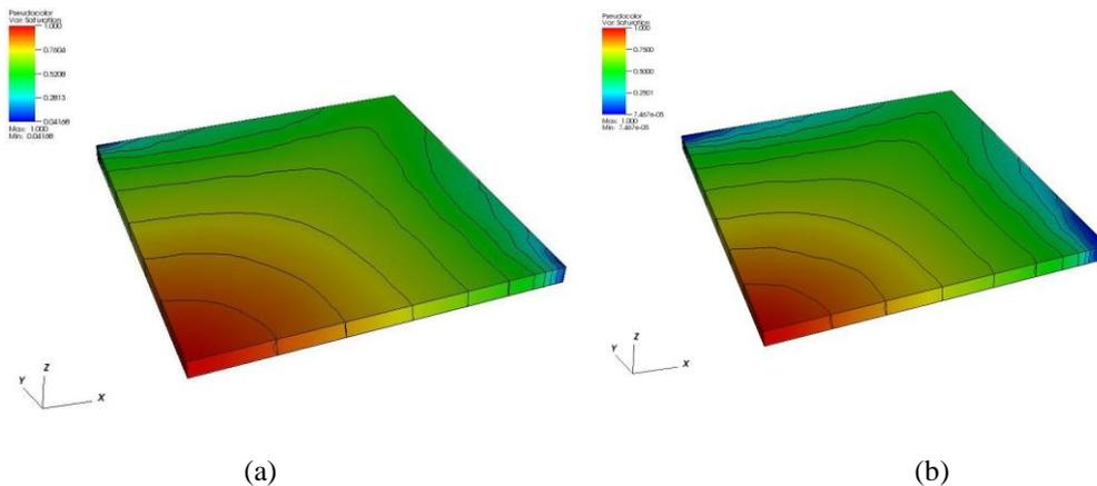
Figure 2.  $\frac{1}{4}$  homogeneous five-spot problem: a) Saturation field obtained with the classical IMPES method at  $t=1.0$  PVI; b) Saturation field obtained with the MIMPES method at  $t=1.0$  PVI, with DVTOL= $10^{-1}$ .
