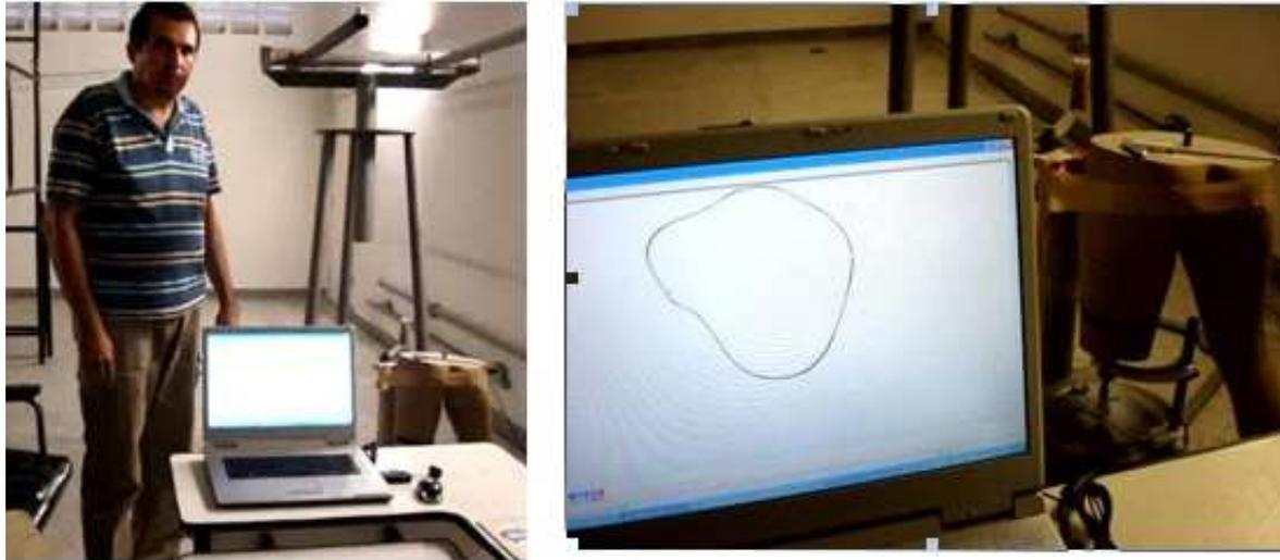
Figure 4. Capturing a Cross Section of a Mannequin's Residual Limb via Pen Tablet to Test the Electronic Interface
