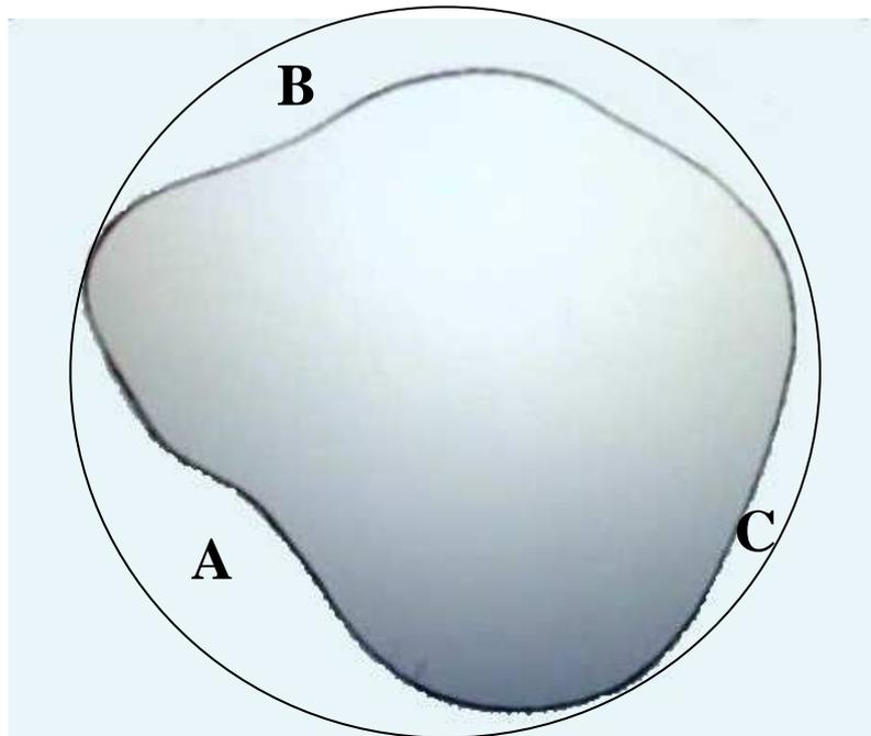
Figure 5. Comparison between a circle obtained by using ordinary tape and the profile from the developed equipment
