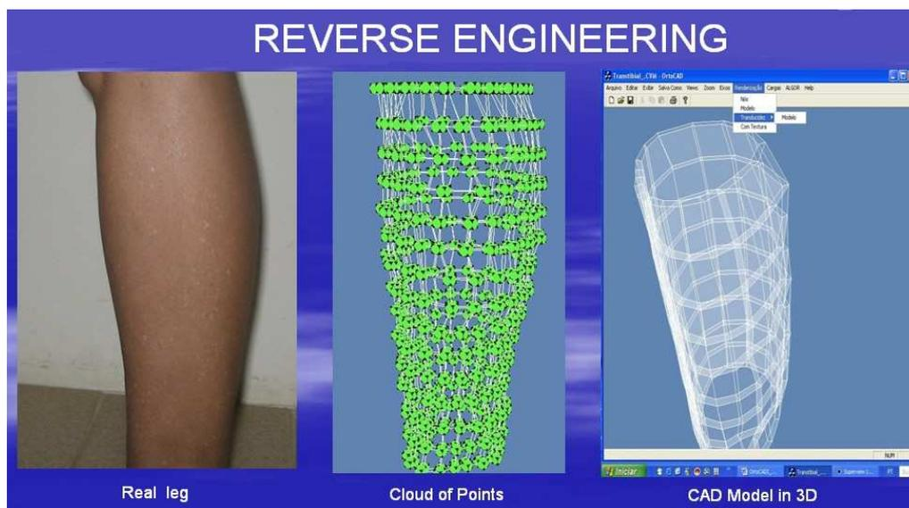
Figure 3. Applying Reverse Engineering through the Electro-Mechanic 3D Scanner and OrtoCAD (Pereira, 2007)
