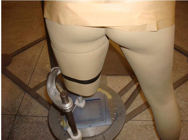
Figure 10 - The Pen Tablet being used to record a mannequin's residual limb (Digital Mode)
