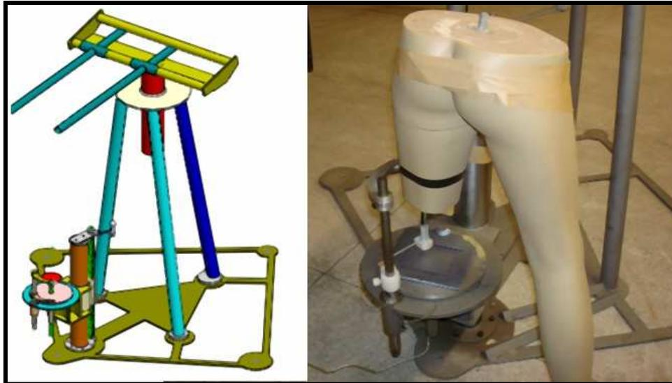
Figure 2. The Electro-Mechanic 3D Scanner (CAD model /Left and Real Device plus Mannequin /Right)
