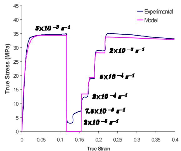
Figure 11a-b: Step Test curve from Del Valle 2005 and model for a magnesium alloy AZ31 at 375 °C
