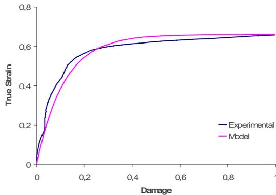
Figure 8: Corrected damage curve. Model and experiment.  $\dot{\epsilon}_1 = 0,0003 \text{ (1/sec)}$ .
