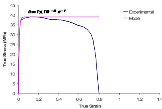
Figure 3: Stress-strain curve and model curve for  $\dot{\epsilon}_2 = 0,01$  (1/sec)
