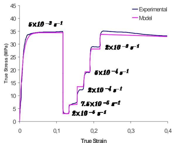
Figure 12a-b: Step Test curve from Del Valle 2005 and model curve for a magnesium alloy AZ31 at 375 °C
