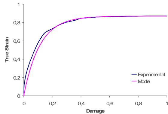
Figure 9: Corrected damage curve. Model and experiment.  $\dot{\epsilon}_2 = 0,01 \text{ (1/sec)}$ .
