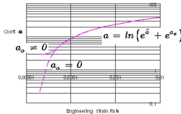
Figure 1: Variation of coefficient  $a$  with  $a_o = 0$  and  $a_o \neq 0$  for a magnesium alloy AZ31 at 375 °C
