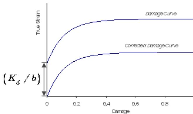
Figure 6: Damage curve and corrected damage curve obtained from a tensile test with constant engineering stress rate.
