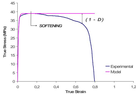
Figure 5: Experimental identification of the auxiliary variable  $D$ .
