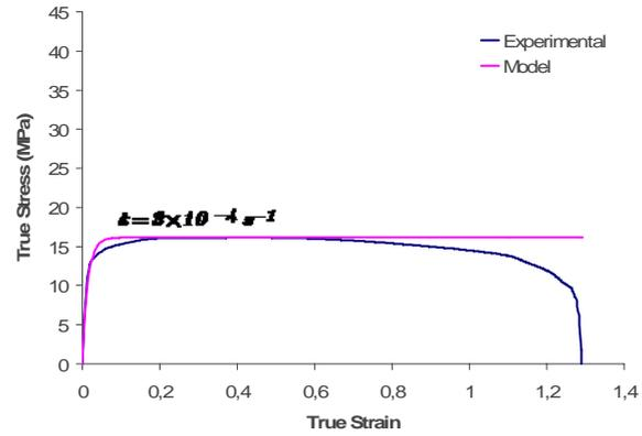
Figure 4: Stress-strain and model curve for  $\dot{\epsilon}_1 = 0,0003$  (1/sec)
