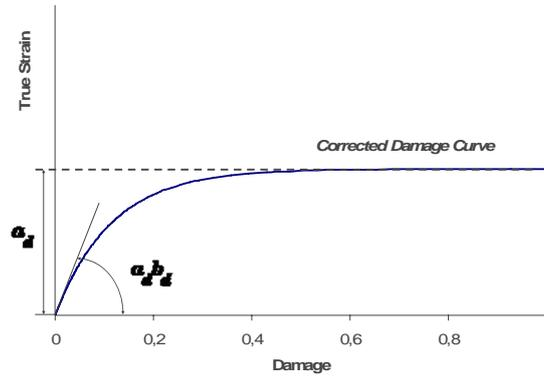
Figure 7: Identification of the parameters  $a_d$  and  $b_d$  from the true stress vs true strain curve
