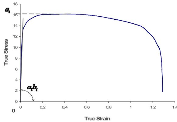
Figure 2: Identification of parameters  $a_i$  and  $b_i$  from the true stress vs true strain curve
