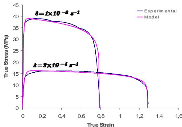
Figure 10: Stress-strain curve for  $\dot{\epsilon}_1 = 0,0003 \text{ (1/sec)}$  and  $\dot{\epsilon}_2 = 0,01 \text{ (1/sec)}$  for a magnesium alloy AZ31B-F at 375 °C
