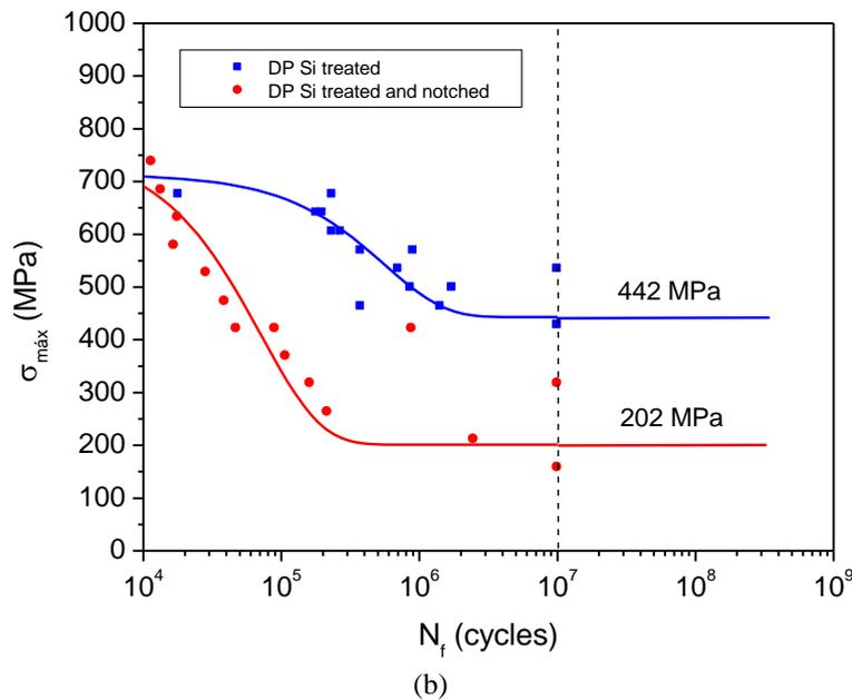
Figure 6. S-N curves for (a) DP-Cr steel and (b) DP-Si steel prestrained and baked, smooth and notched specimens
