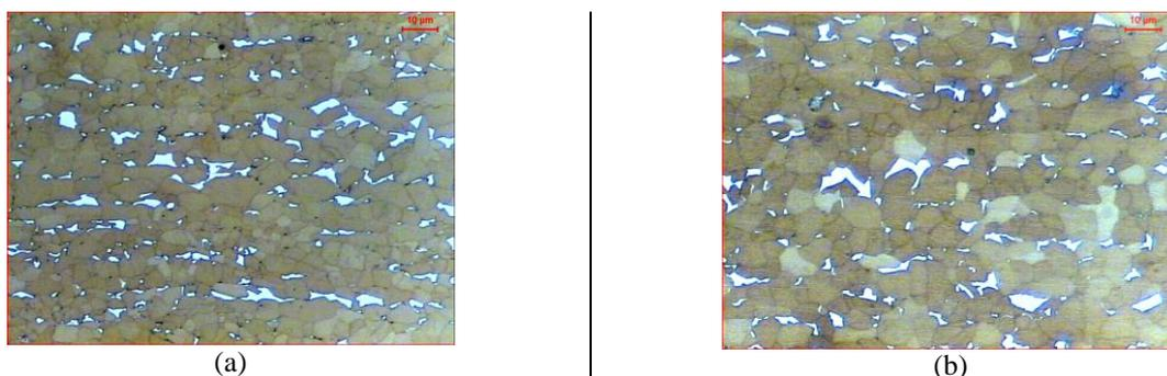
Figure 2. Optical microstructure of the two dual-phase steel, consisting of ferrite (dark) surrounding martensite (white) Transverse direction. LePera's etching. 1000X. (a) DP-Cr steel; (b) DP-Si steel
