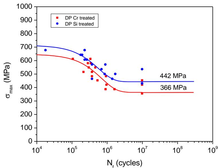
Figure 3. S-N curves for the two steels treated (prestrained and baked), smooth specimens
