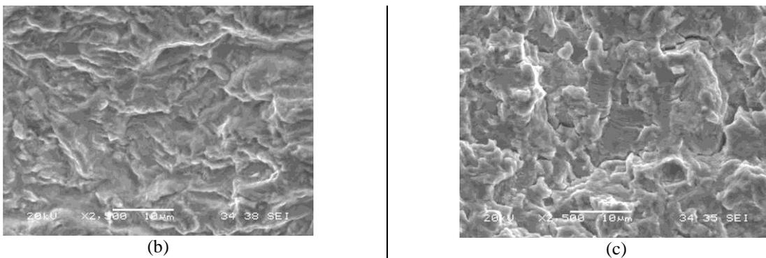
Figure 5. SEM fractography of fatigue surface from the DP-Si steel, (a) general view, 100X; (b) crack origin and crack growth by facets, 2500X; (c) crack growth by striations and secondary cracks, 2500X; arrow indicates the crack growth direction
