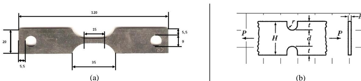
Figure 1. (a) Geometry and dimensions (in mm) of specimens for fatigue tests
