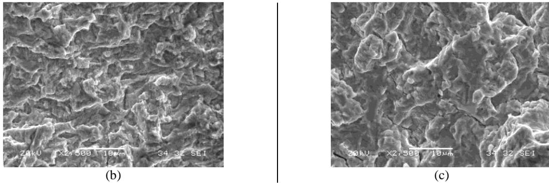
Figure 4. SEM fractography of fatigue surface from the DP-Cr steel, (a) general view, 100X; (b) crack origin and crack growth by facets, 2500X; (c) crack growth by striations and secondary cracks, 2500X; arrow indicates the crack growth direction
