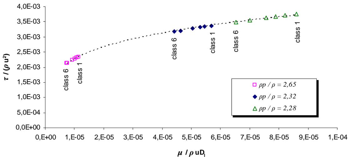
Figure 8. Dimensionless minimum shear stress in function of Reynolds number
