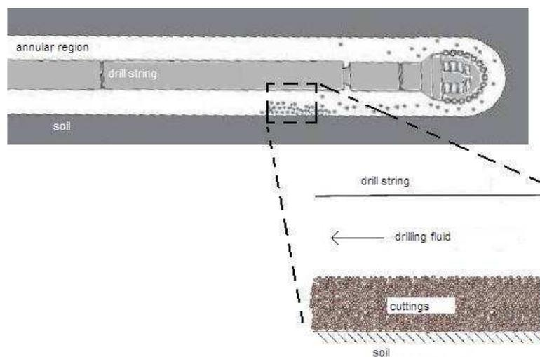
Figure 1. Drilling of high inclination
