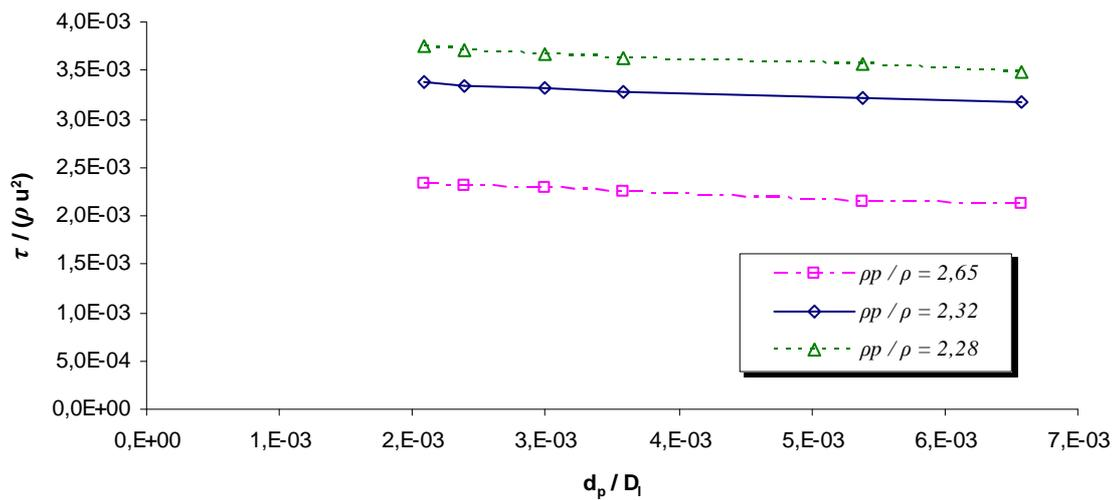
Figure 6. Dimensionless variation of threshold shear stress for particle diameter
