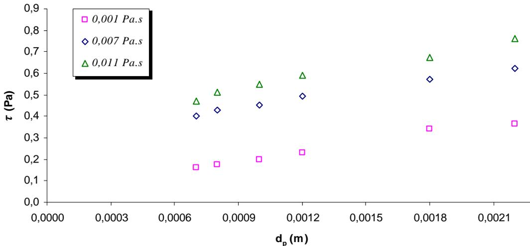
Figure 5. Influence of particle diameter at the threshold shear stress
