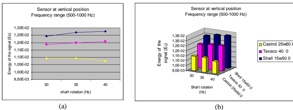
Figure 4. Energy of the Signal for the Lubricants without contamination from 550 to 1000 Hz in the vertical position. (a) Linear representation, (b) bar representation
