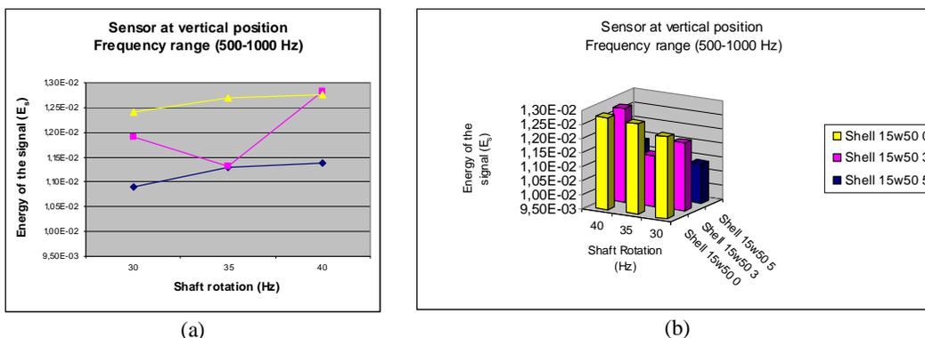
Figure 6. Energy of the Signal for the Shell lubricants without and with two contamination grades from 500 to 1000 Hz measured in the vertical position. (a) Linear representation, (b) bar representation
