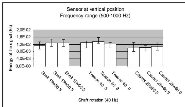
Figure 11. Energy of the signal for the three lubricant brands with and without two contaminant grades from 500-1000 Hz measured in vertical position at 40 Hz
