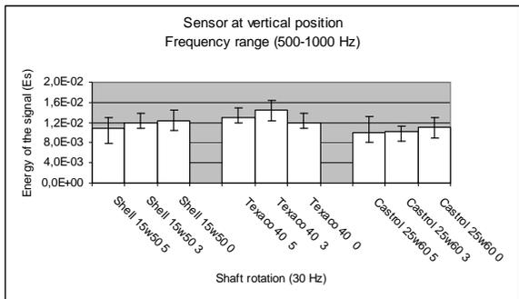
Figure 9. Energy of the signal for the three lubricant brands with and without two contaminant grades from 500-1000 Hz measured in vertical position at 30 Hz
