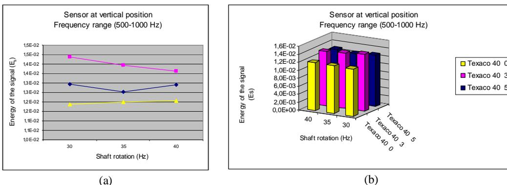
Figure 7. Energy of the Signal for the Texaco lubricants without and with two contamination grades from 500 to 1000 Hz measured in the vertical position. (a) Linear representation, (b) bar representation
