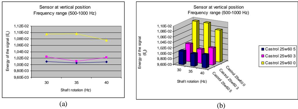
Figure 8. Energy of the Signal for the Castrol lubricants without and with two contamination grades from 500 to 1000 Hz measured in the vertical position. (a) Linear representation, (b) bar representation
