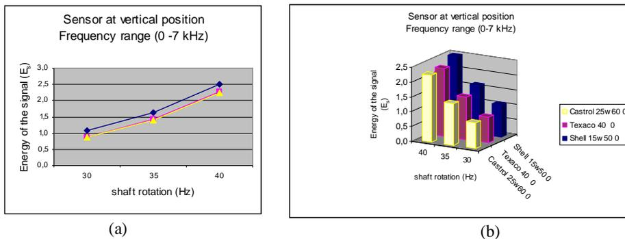
Figure 2. Energy of the Signal for the Lubricants without contamination from 0 to 7 k Hz in the vertical position. (a) Linear representation, (b) bar representation
