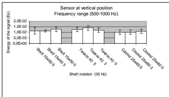
Figure 10. Energy of the signal for the three lubricant brands with and without two contaminant grades from 500-1000 Hz measured in vertical position at 35 Hz
