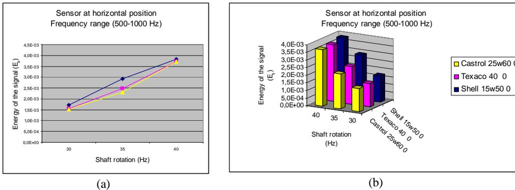
Figure 5. Energy of the Signal for the Lubricants without contamination from 500 to 1000 Hz in the horizontal position. (a) Linear representation, (b) bar representation
