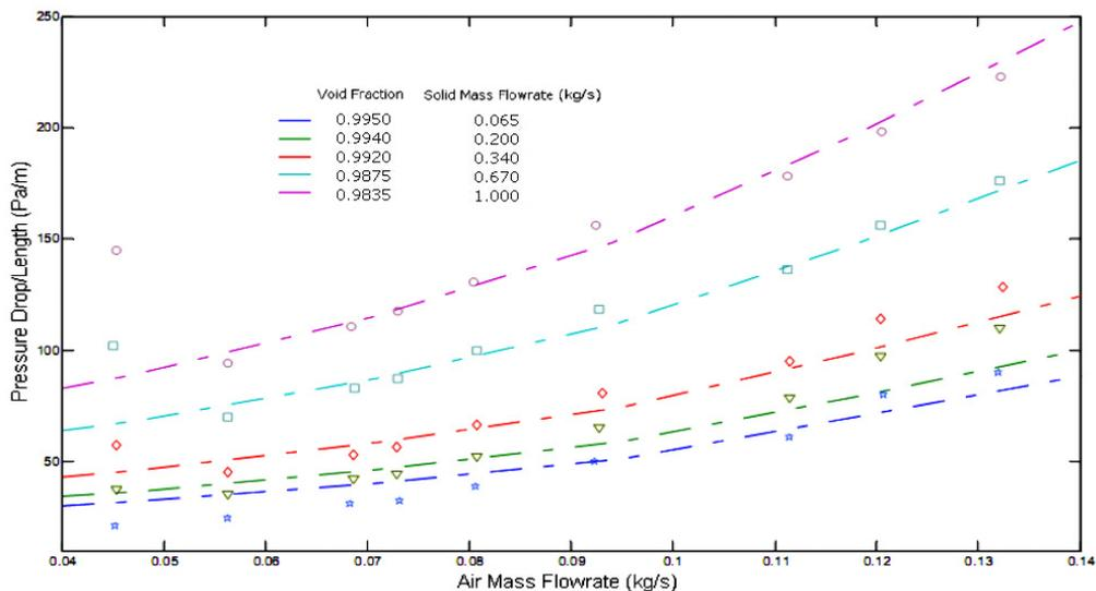
Figure 5. Comparison of the pressure drops with Herbreteau and Bouard's experimental data for 0.203 mm glass beads. Model A.
