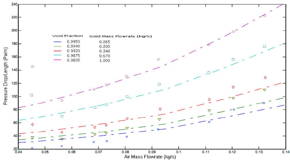
Figure 7. Comparison of the pressure drops with Herbreteau and Bouard's experimental data for 0.203 mm glass beads. Model C.
