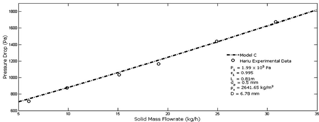
Figure 3 – Comparison of the relative-velocity-model pressure drops with Hariu and Molstad's experimental data for an assumed inlet void fraction of  $0.955$ .
