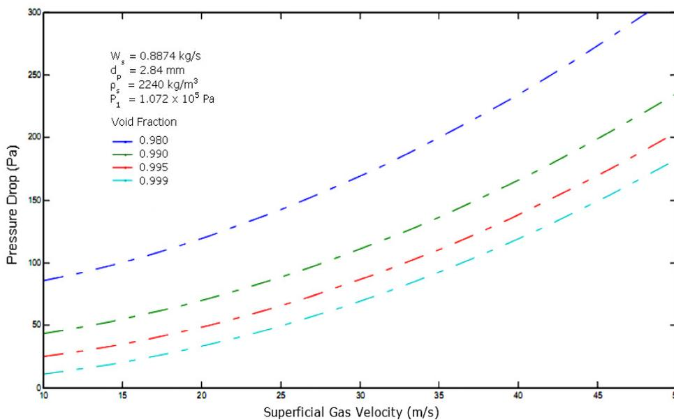
Figure 9. The effect of initial gas volume fraction on the pressure drop for the flow of a solid-gas mixture through a horizontal pipe calculated by using the relative velocity model.
