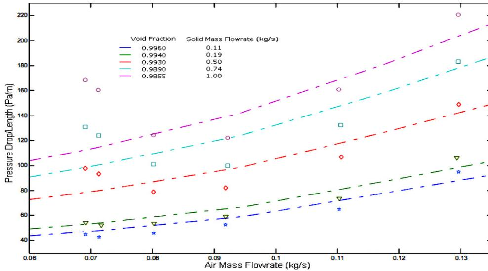
Figure 4. Comparison of the pressure drops with Herbreteau and Bouard's experimental data for 0.035 mm glass beads. Model A.
