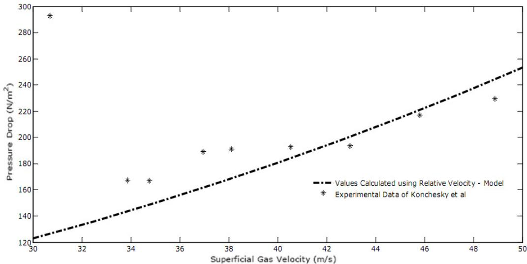
Figure 2 – Drop pressure versus Superficial Gas Velocity.
