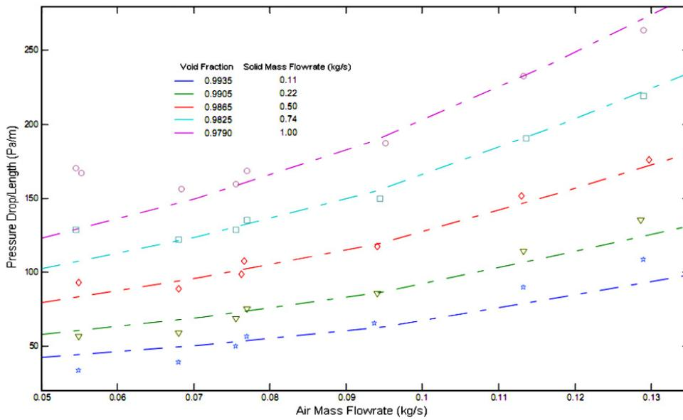
Figure 8. Comparison of the pressure drops with Herbretau and Bouard’s experimental data for 0.340 mm glass beads. Model A.
