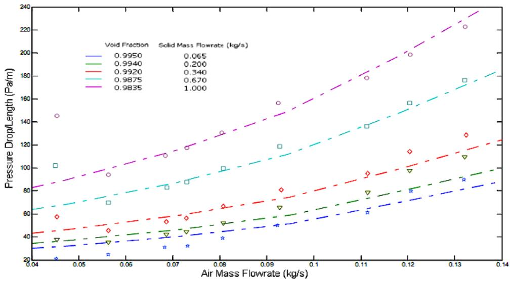
Figure 6. Comparison of the pressure drops with Herbreteau and Bouard's experimental data for 0.203 mm glass beads. Model B.
