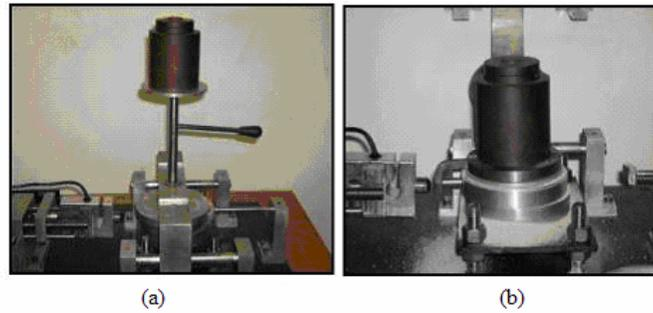
Figure 4 - Jenike Cell built at the laboratory, (a) sample under torsion (b) Shear process.
