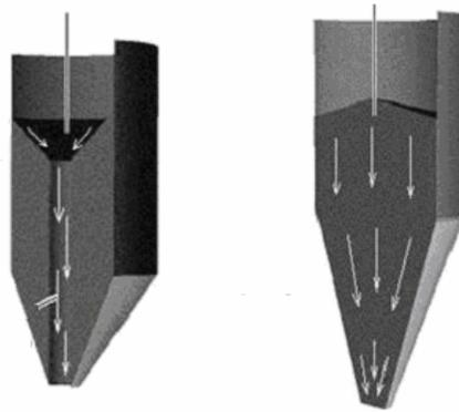
Figure 1 - Discharge patterns from the silos: (right) mass flow; (left) funnel flow.
