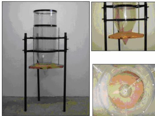
Figure 5 – Silo prototypes.
