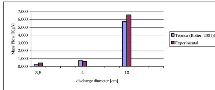
Figure 8 – Mass flow rate for kaolin.
