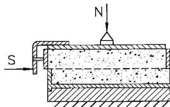
Figure 3 - Material submitted to the shear process (AST, 1997).
