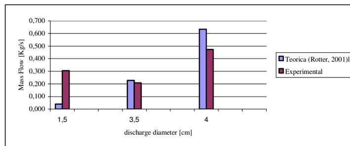
Figure 9 - Mass flow rate for alumina.
