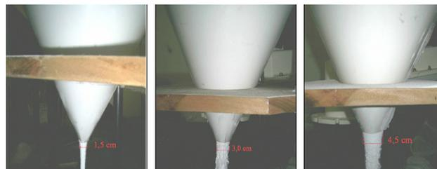
Figure 7 - Different drainage conditions in different discharge diameters for Alumina.
