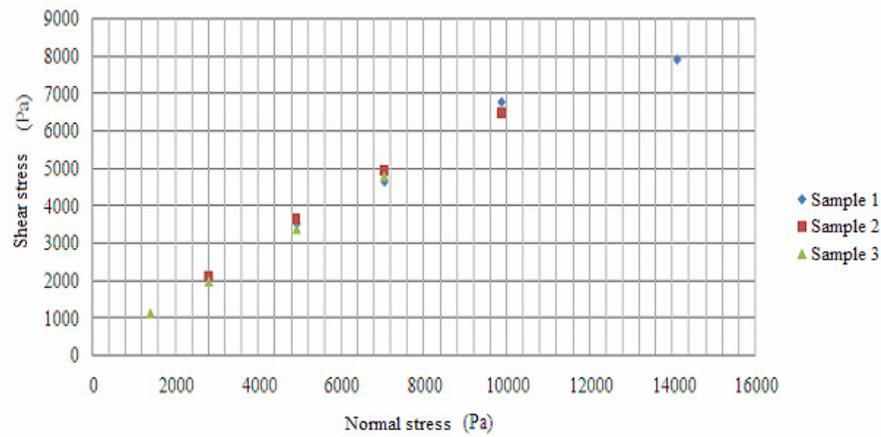
Figure 6 – Fluency curve for Alumina.
