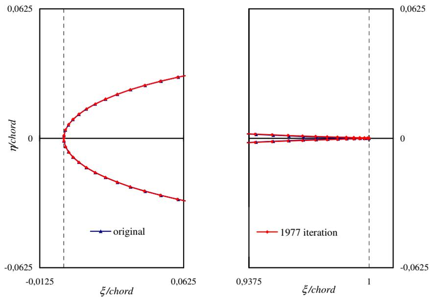
Figure 3. Final geometries of the leading and trailing edges of the symmetric Joukowski airfoil
