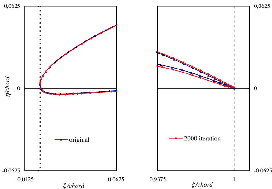
Figure 7. Final geometries of the leading and trailing edges of the non symmetric airfoil NACA 65-1210
