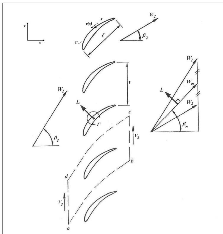
Figure 1. Geometry of cascade and triangles of velocity
