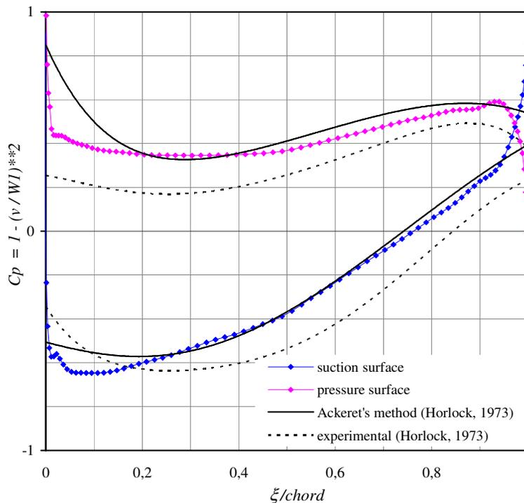
Figure 8. Pressure coefficient distribution over the surfaces of the airfoil NACA 65-1210 in cascade (stagger  $\chi = 30^\circ$ , pitch chord ratio  $t/l = 1,0$ ) for  $\beta_1 = 45^\circ$ ; the present code results  $\beta_2 = 23,5^\circ$  with  $2N = 160$  control points
