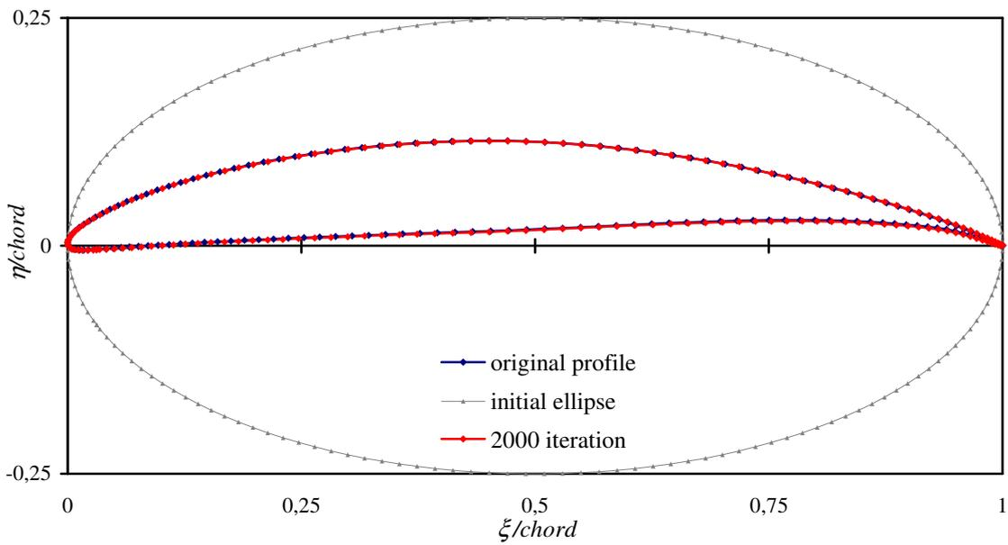
Figure 6. Design of the NACA 65-1210 airfoil ( $2N = 160$ )
