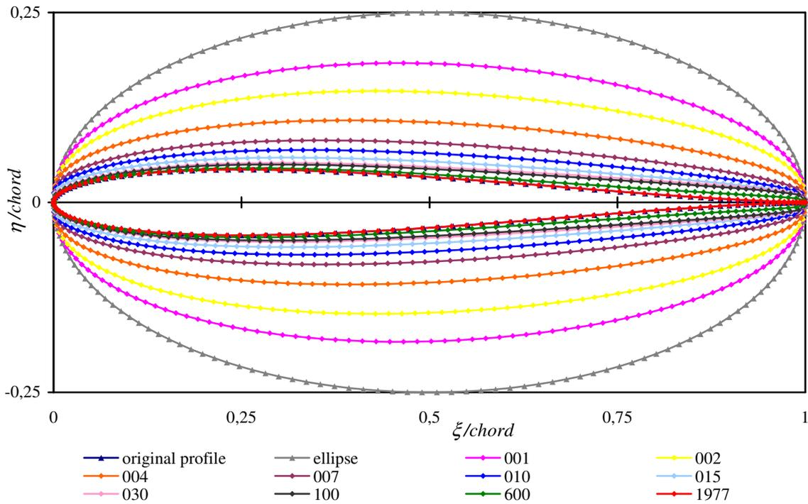
Figure 2. Evolution of the calculated foil shapes of a Joukowski symmetric airfoil ( $2N = 160$ )
