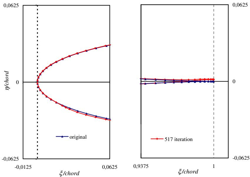
Figure 5. Final geometries of the leading and trailing edges of the symmetric Joukowski airfoil ( $\beta_\infty = 10^\circ$ )
