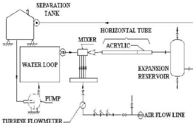
Figure 1. Schematic of air-water test section
