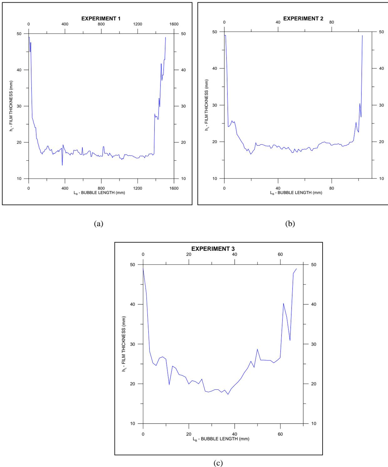
Figure 4. Wave bubble shape from (a) Experiment 1 (b) Experiment 2 (c) Experiment 3
