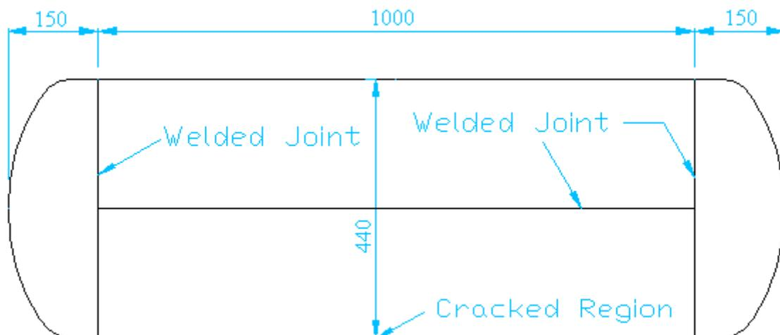
Figure 1. Dimensions of the pressure vessel
