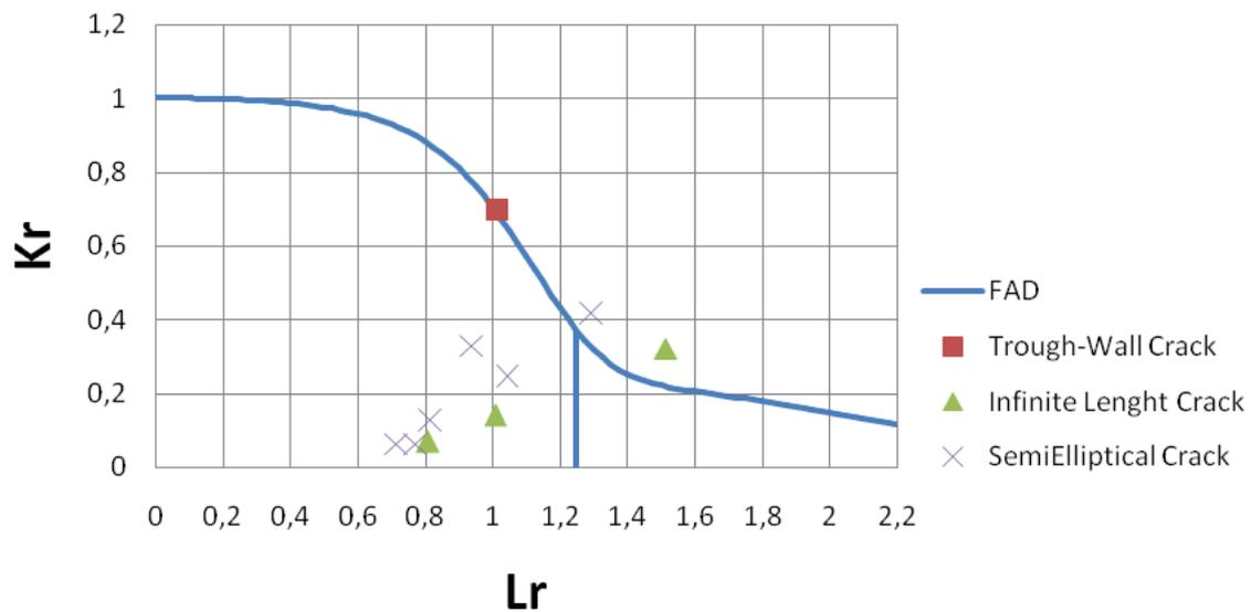
Figure 5. Results plotted in FAD
