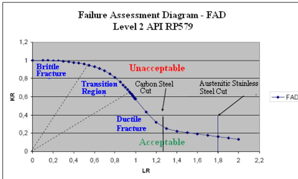
Figure 4. Failure Assessment Diagram
