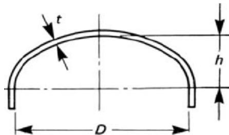
Figure 3. Main Dimensions of Elliptical Heads
