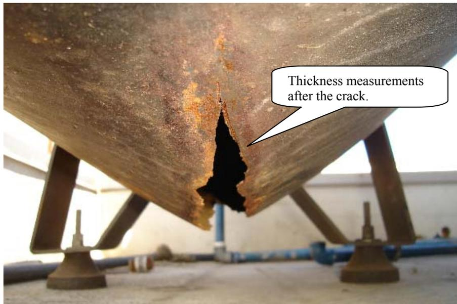
Figure 2. The pressure vessel after the failure
