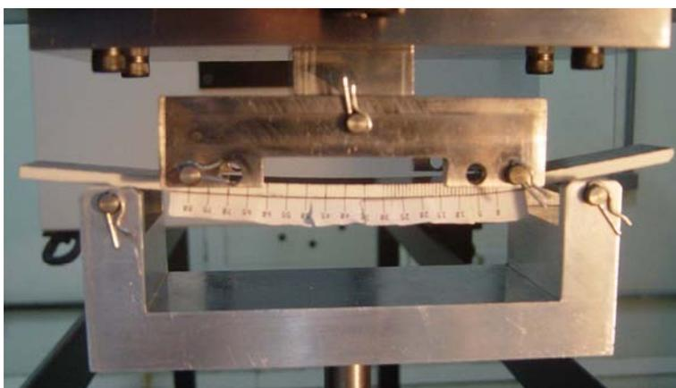
Figure 7. MMB test apparatus
