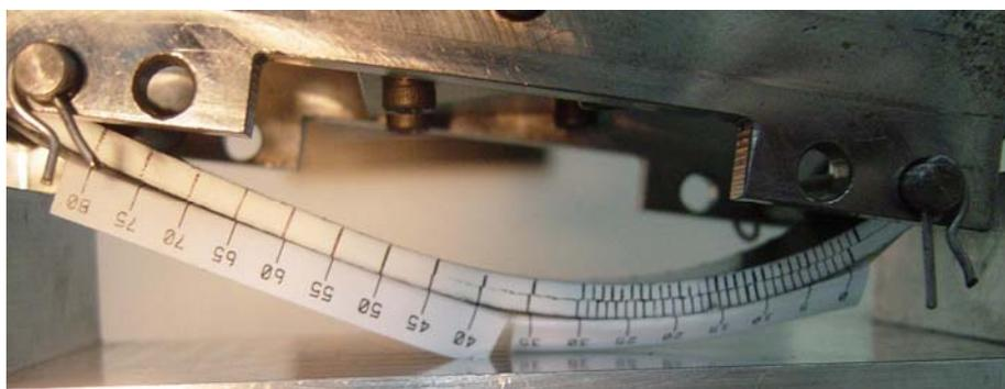
Figure 10. Large deformations on 4ENF test
