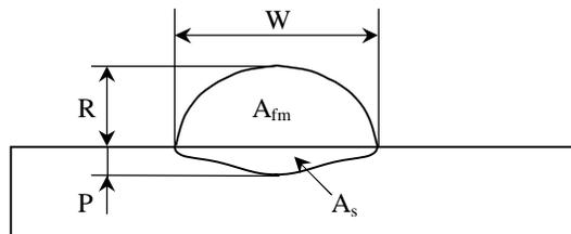
Figure 2. Weld bead geometry.
