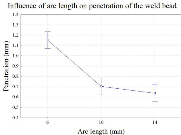
Figure 7. Influence of arc length on penetration of weld bead.
