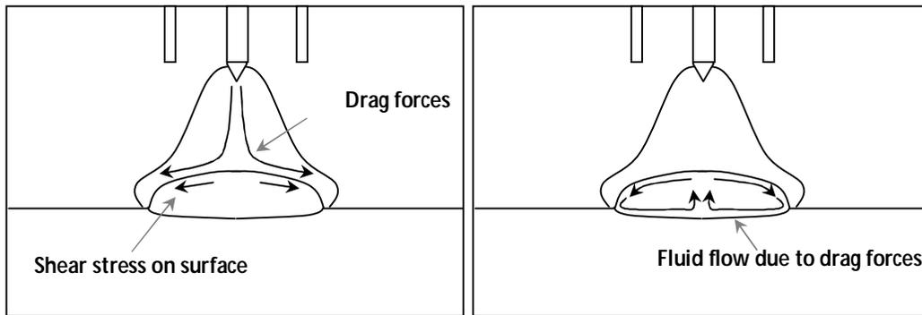
Figure 9. Weld pool convection due to drag forces.
