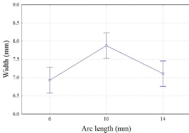
Figure 6. Influence of arc length on width of weld bead.
