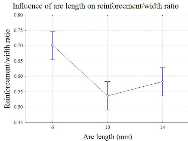
Figure 9. Influence of arc length on reinforcement/width ratio.
