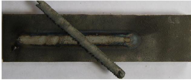
Figure 4. Sample welded with low heat input and 10 mm arc length.
