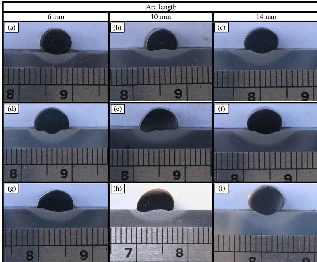
Figure 3. Transverse cross section of the weld bead welded. (a), (b) and (c)  $E = 9.6$  kJ/cm; (d), (e) and (f)  $E = 12.3$  kJ/cm; (g), (h) and (i)  $E = 14.8$  kJ/cm.
