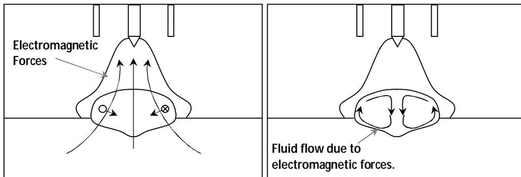
Figure 8. Weld pool convection due to electromagnetic forces.
