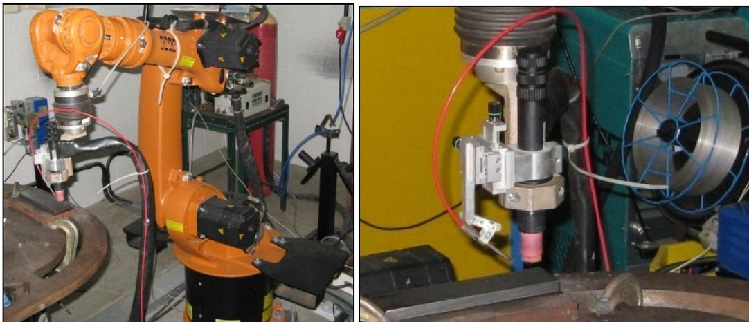
Figure 1. (a) Robotic system. (b) detail of wire feeder guide and torch.
