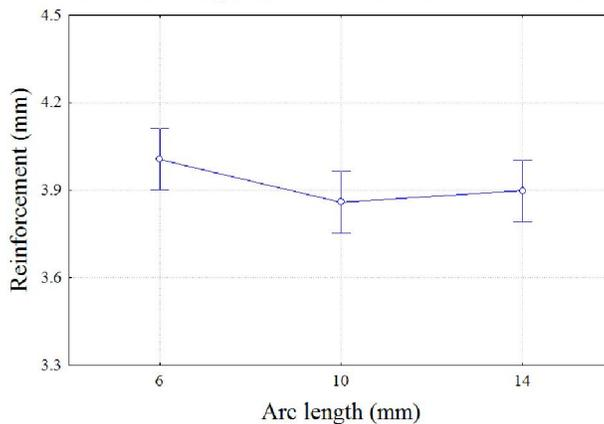
Figure 5. Influence of arc length on reinforcement of weld bead.
