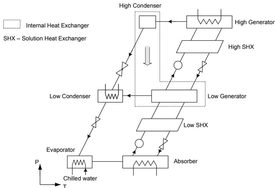
Figure 2. Parallel flow double-effect water/lithium bromide chiller Dühring chart schematic.
