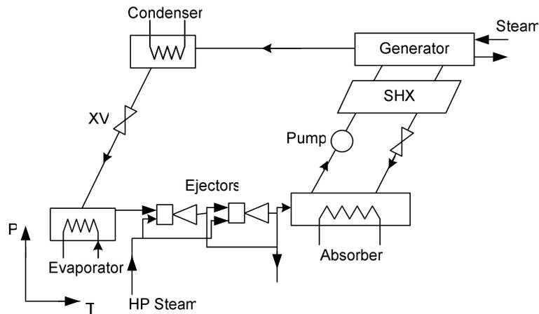
Figure 3. Absorption-ejecto compression refrigeration system Dühring chart schematic.
