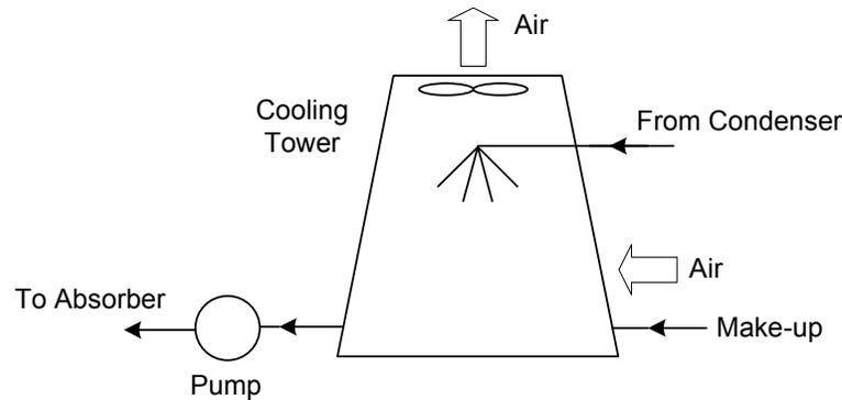
Figure 5. Cooling system for absorption refrigeration systems.
