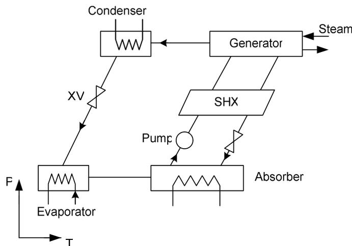
Figure 1. Single effect water/lithium bromide absorption chiller Dühring chart schematic.
