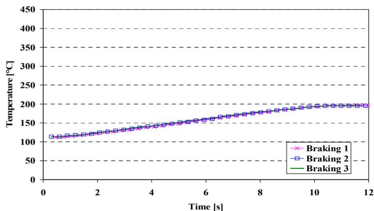
Figure 3.2 – Temperature curves measured by thermocouple (slipping velocity of 7.4 to 3.7 m/s, torque of 47 Nm and material B).
