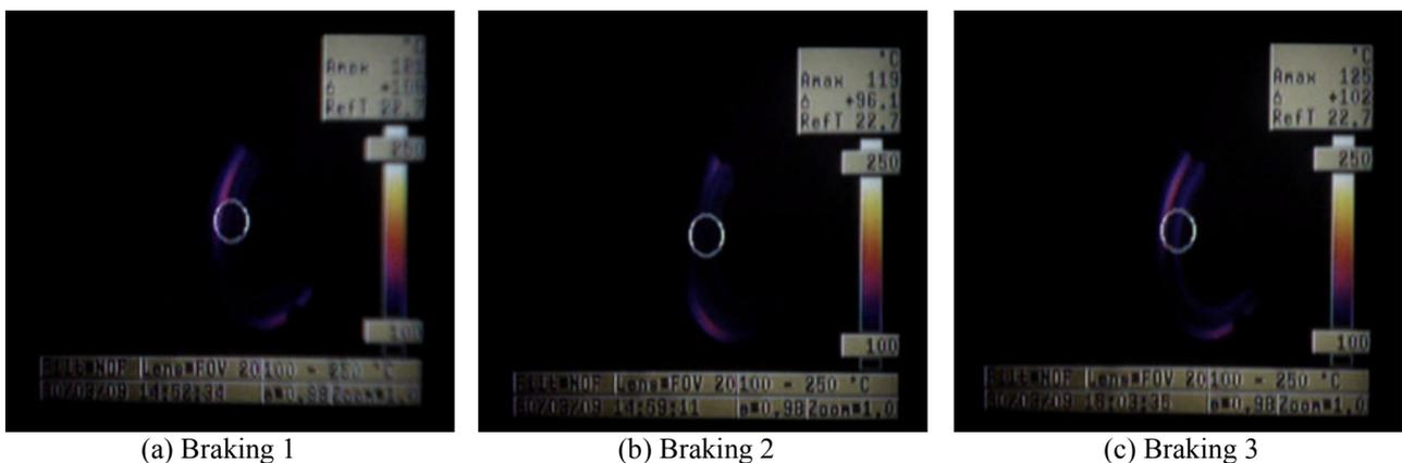
Figure 3.9 – Thermographic images produced at velocity of 16.6 to 13.8 m/s and torque of 47 Nm (material A).
