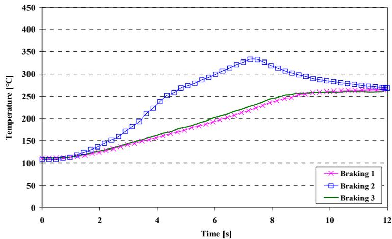
Figure 3.8 – Temperature curves measured by thermocouple (slipping velocity of 16.6 to 13.8 m/s, torque of 47 Nm and material B).
