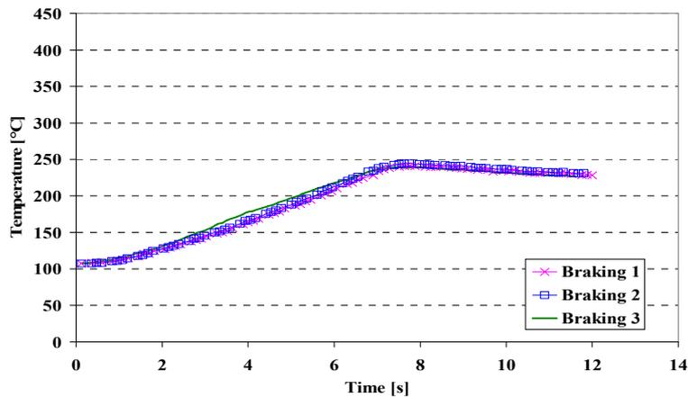
Figure 3.10 – Temperature curves measured by thermocouple (slipping velocity of 16.6 to 13.8 m/s, torque of 47 Nm and material A).
