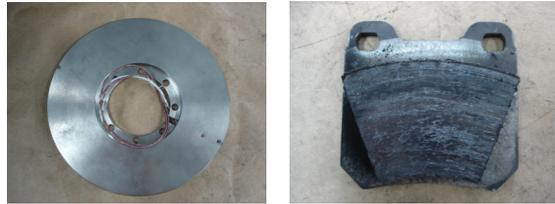
Figure 2.1 – Friction pair tested.
