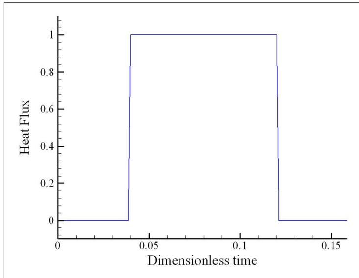
Figure 3.a – Exact heat flux imposed in the simulated experimental data in dimensionless form
