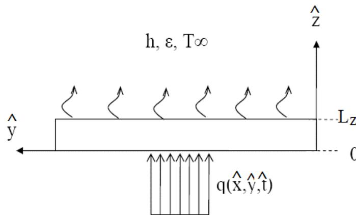
Figure 1.b – Lateral view of the heated thin plate.
