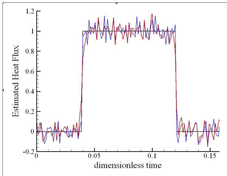
Figure 5 – Comparison between the exact and the estimated heat flux, with 120 parameters for a search step of 0.001 (red curve) and 0.005 (blue curve)
