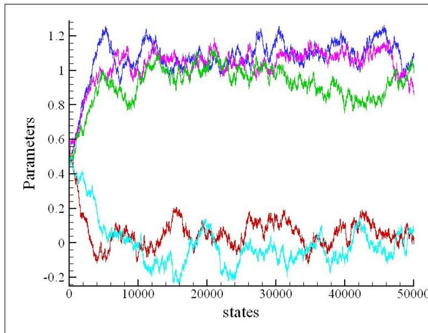
Figure 4.b - Markov chain evolutions for search step of 0.005, for 5 different parameters
