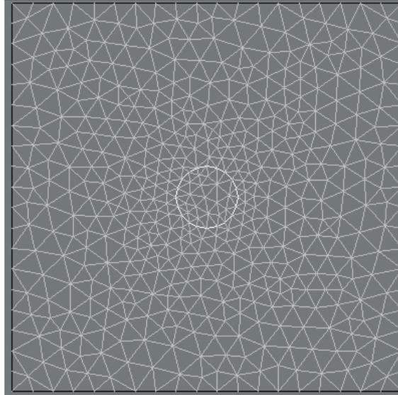
Figure 2 - Mesh of plate surface into triangular elements used to the code implementation based on FEM.
