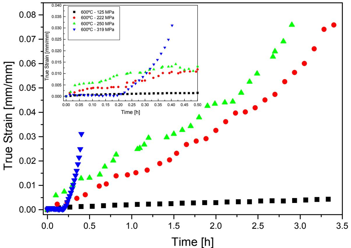
Figure 9. Creep curves of the Ti-6Al-4V at 600°C and 125, 222, 250 and 319 MPa with Widmanstätten structure.
