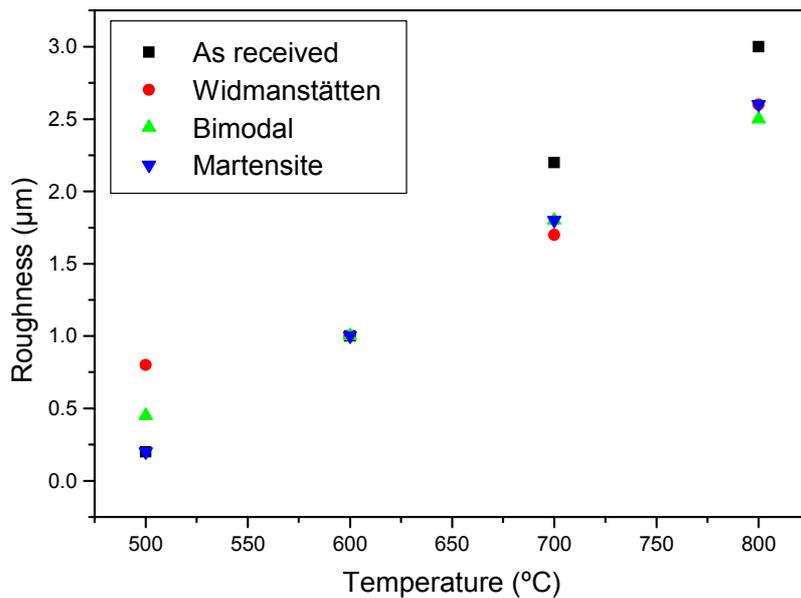
Figure 6. Roughness measures of the microstructures obtained by heat treatment as a function of oxidation temperature.
