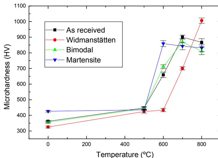
Figure 5. Micro hardness measures of the microstructures obtained by heat treatment.
