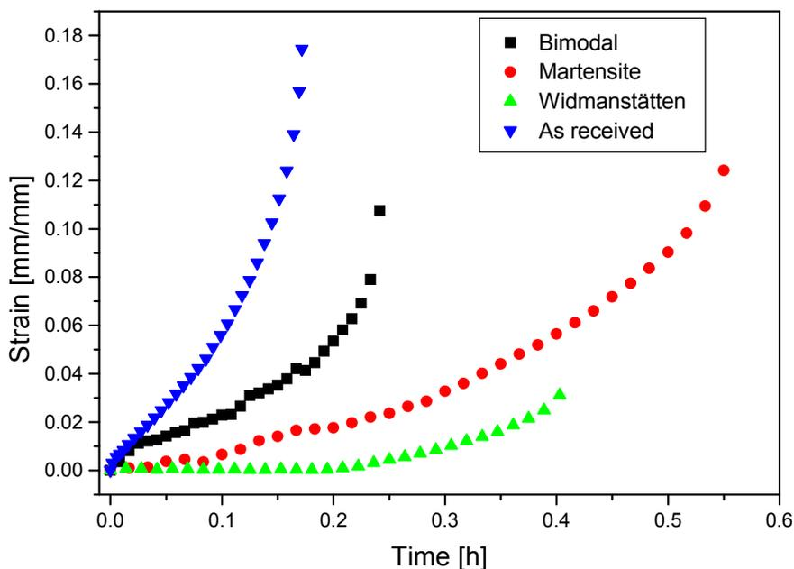
Figure 8. Creep curves of the Ti-6Al-4V alloy at 600°C and 319 MPa, as received and with structures: Widmanstätten, Martensite and Bimodal.
