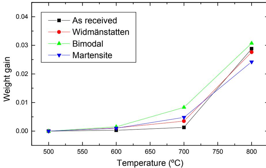
Figure 4. Weight gain measures of microstructures as a function of oxidation temperature for 48 hours.
