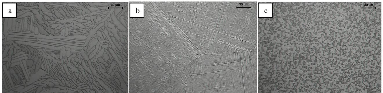
Figure 3. Structures obtained in heat treatments: a) Widmanstätten b) Martensite and c) Bimodal.
