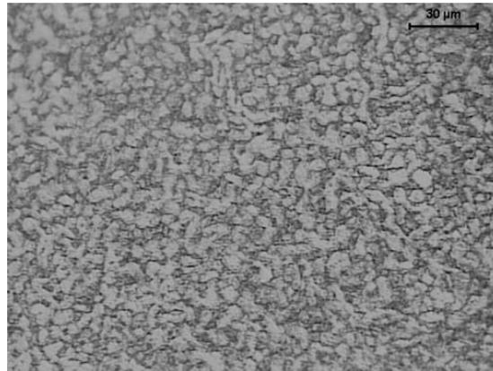
Figure 2. Ti-6Al-4V alloy micrograph as received.
