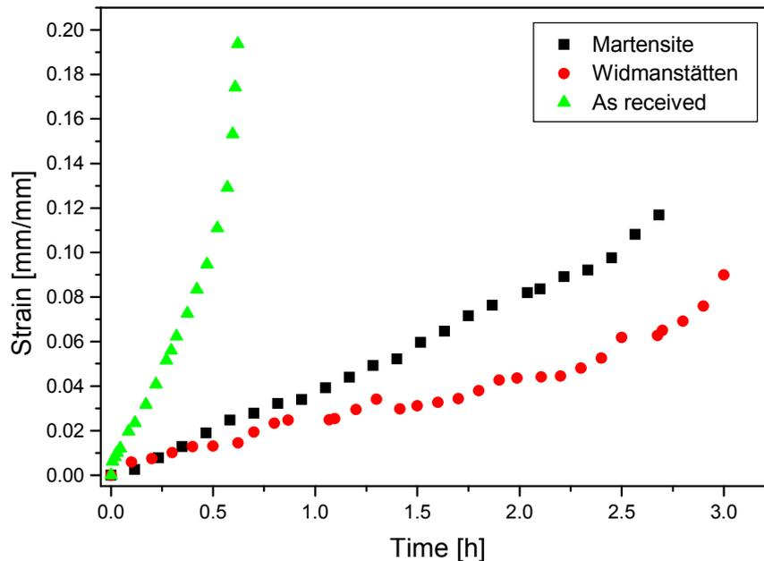
Figure 7. Creep curves of the Ti-6Al-4V alloy at 600 °C and 250 MPa as received and with structures: Martensite and Widmanstätten.
