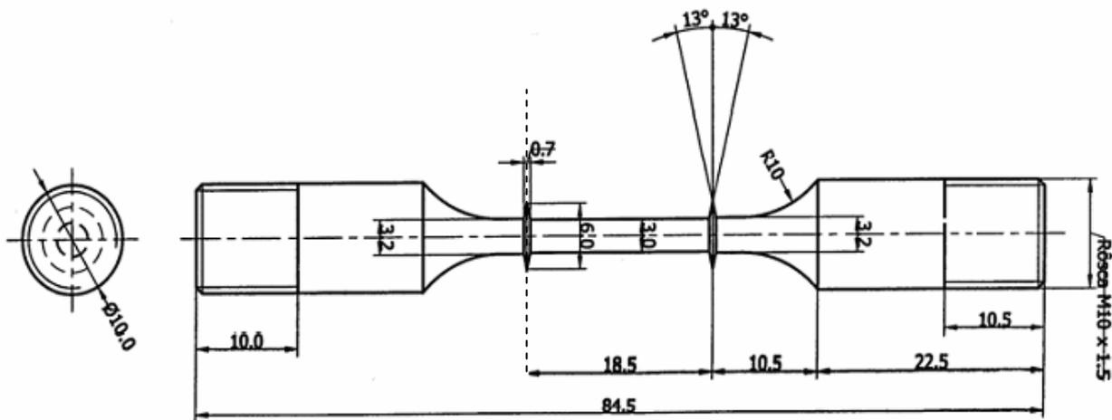
Figure 1. Schematic view of the specimen creep test.
