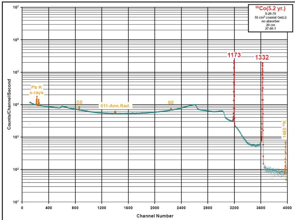
Figure 2. The energy spectrum of the radioisotope Cobalt-60.
