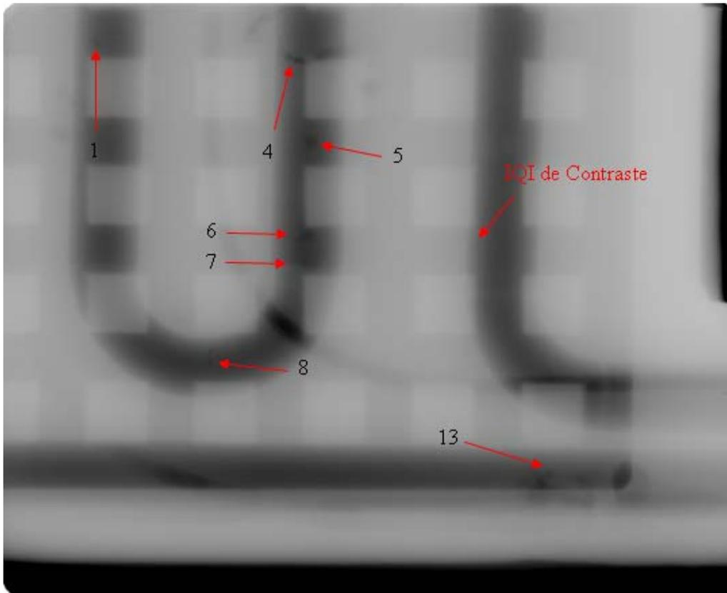
Figure 7. Image obtained with a class 1 film showing discontinuities in the areas of smaller thickness.
