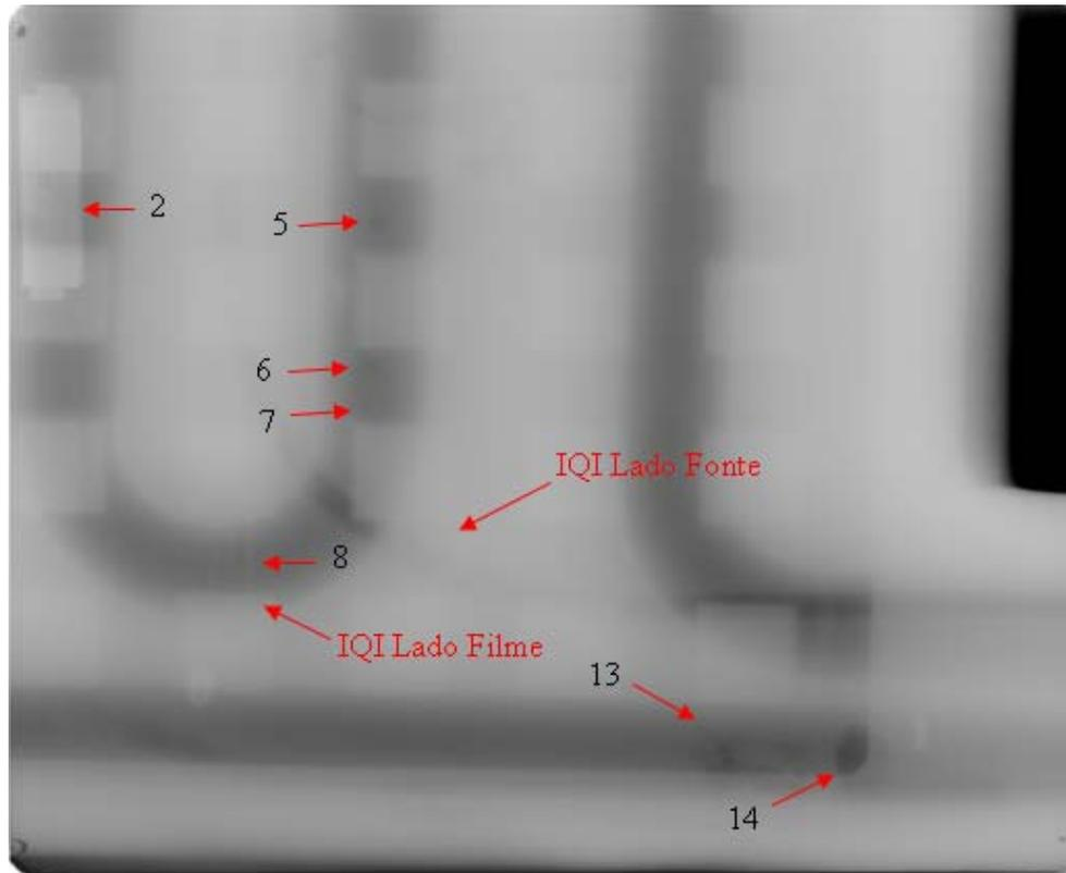
Figure 10. Radiographic image using one film class 2 (simple view).
