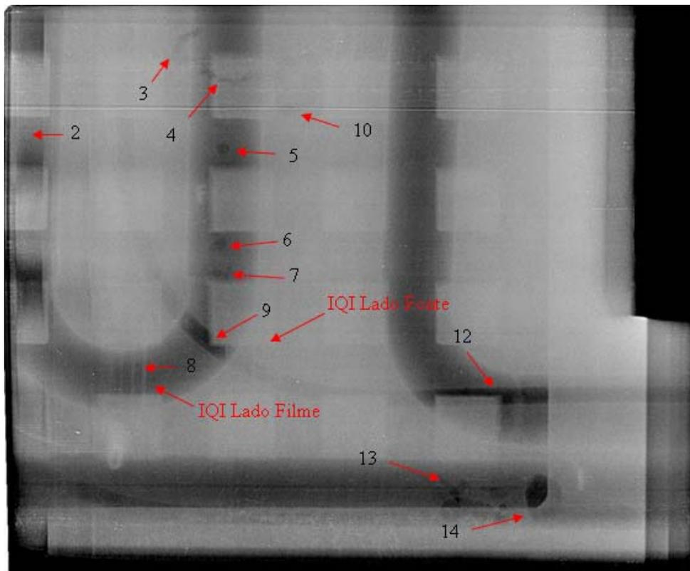
Figure 11. Industrial computed radiography using Cobalt-60.
