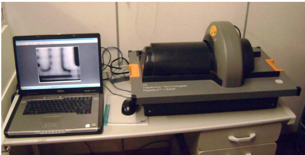
Figure 3. Industrial computed radiography equipment GE CR50P.
