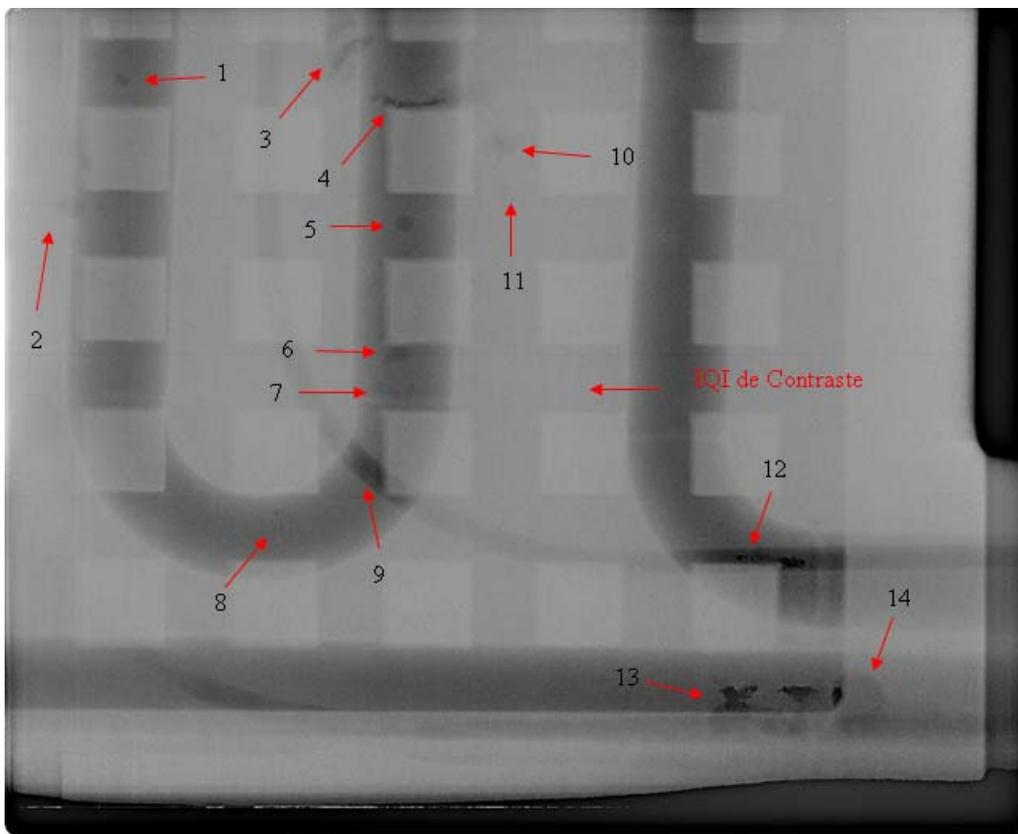
Figure 8. Image obtained by industrial computed radiography with mathematical processing.
