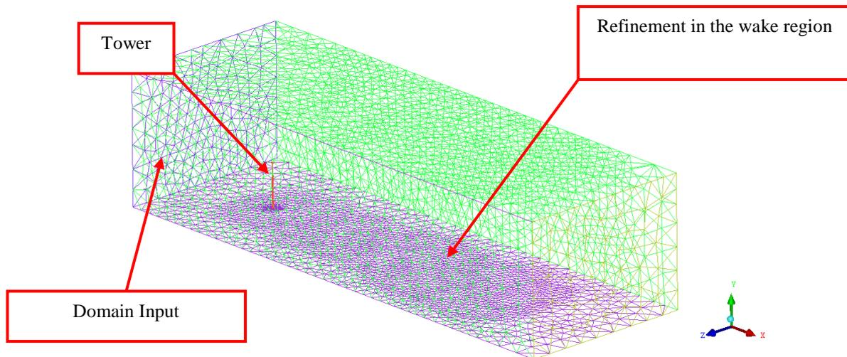
Figure 4. Mesh of the static part of the problem
