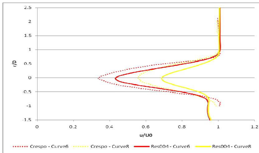
Figure 8. Profiles of averaged velocities “u” for 6 and 8 diameters
