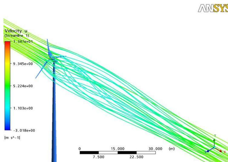
Figure 6. Streamlines on the turbine
