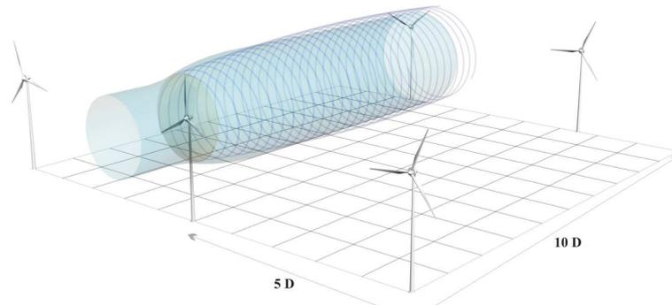
Figure 1. Vortex wake and turbine distance (ATLAS DO POTENCIAL EÓLICO BRASILEIRO, 2001).
