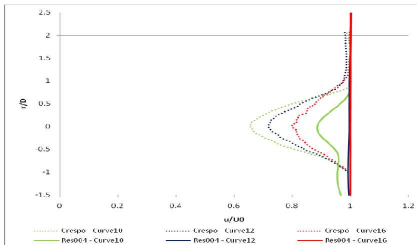
Figure 9. Profiles of averaged velocities “u” for 10, 12 and 16 diameters
