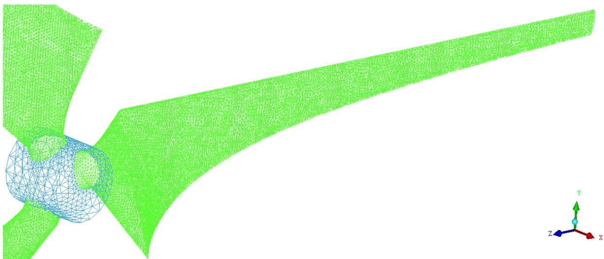
Figure 3. Surface mesh of a rotor blade
