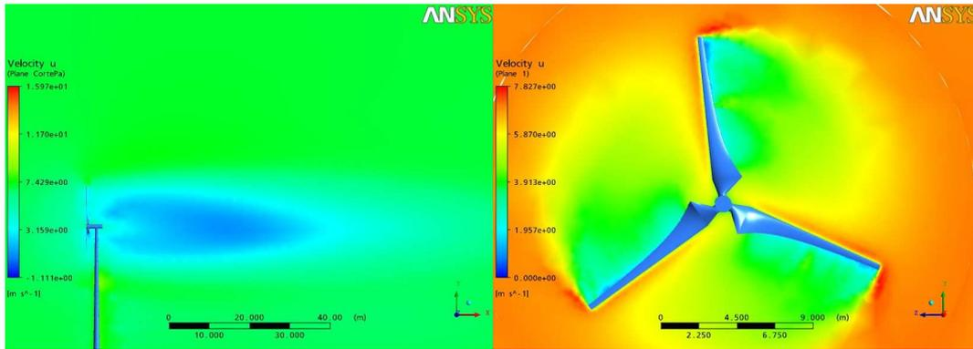
Figure 5. Velocity “u” in the central area (left) and into the rotor of turbine.
