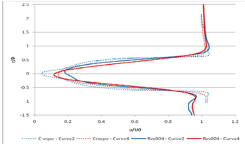
Figure 7. Profiles of averaged velocities “u” for 2 and 4 diameters
