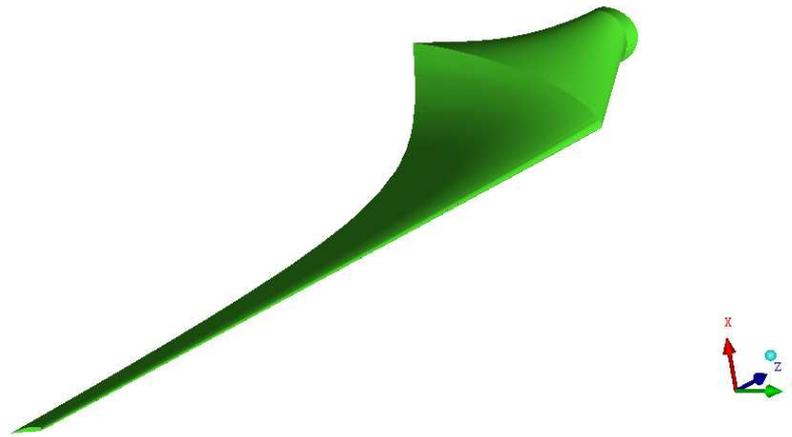
Figure 2. Blade profile generated according to Betz optimal design.
