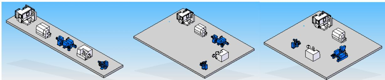
Figure 2. Modeling options for layout in line, in "L" and "U" for 5 machines cell.
