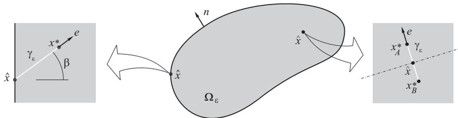
Figure 1. Elastic cracked body represented by the domain  $\Omega_\varepsilon$ .
