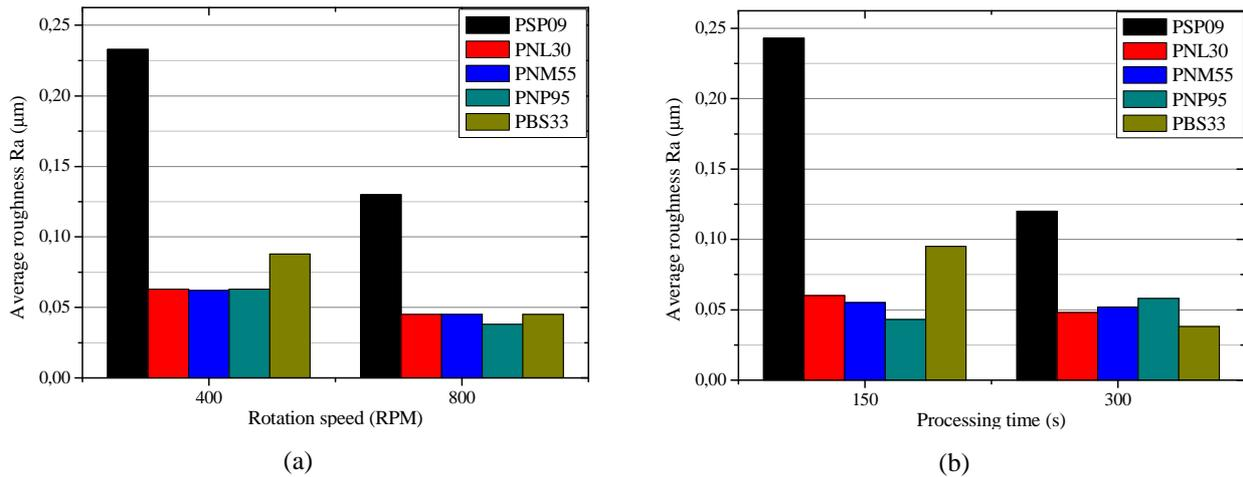
Figure 5. Variation of surface roughness for different oils as a function of: (a) rotation speed; and (b) processing time.
