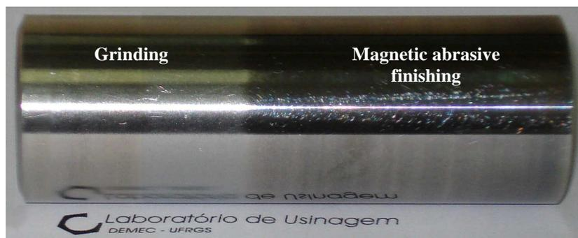
Figure 8. Surface quality obtained through grinding and magnetic abrasive finishing.
