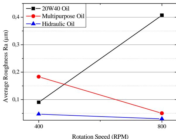
Figure 1. Surface roughness obtained by Amorim, 2008, for different oils at different rotation speeds.
