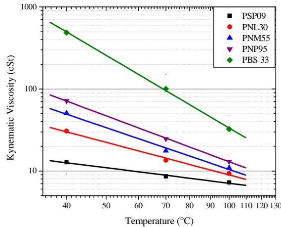
Figure 2. Viscosity as a temperature function for studied oils.
