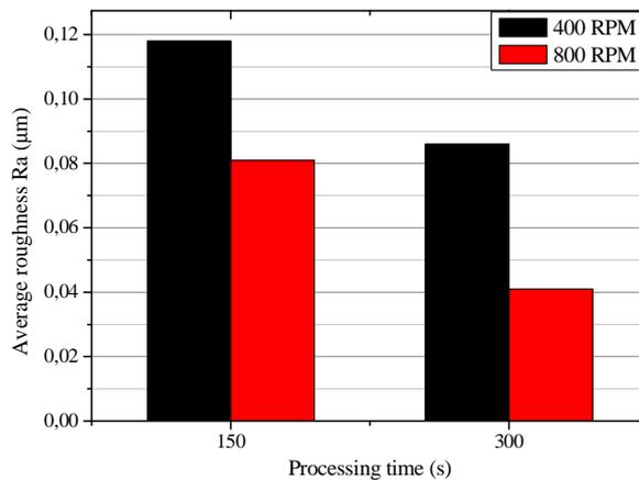
Figure 3. Surface roughness obtained after different processing times.
