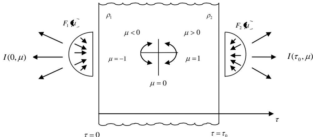
Figure 1 – Schematical representation of one-dimensional homogeneous participating, with inner diffusely reflecting boundary surfaces, subjected to isotropic external radiation
