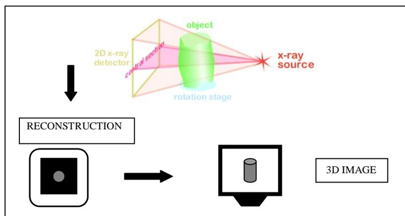
Figure 3: An illustration of the acquisition and reconstruction processes with cross-section to image in  $\mu$ -CT.
