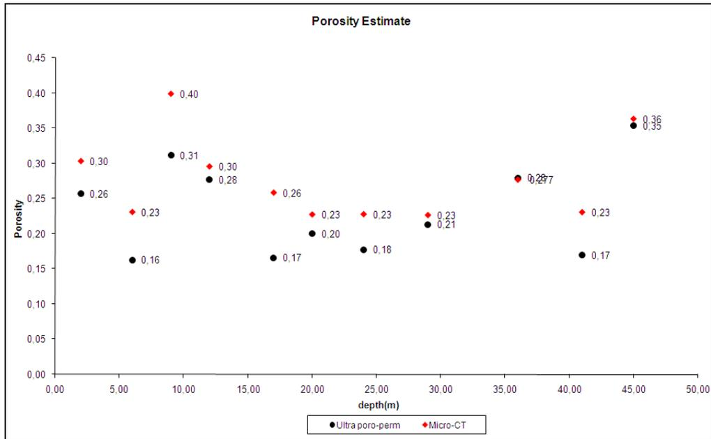
Figure 5: Porosity values of GPR3 well estimate by  $\mu$ -CT and Ultra poro-perm:
