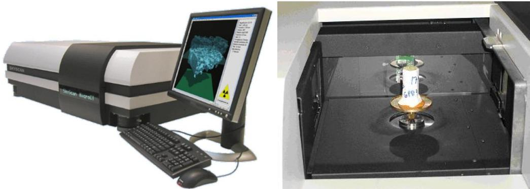
Figure 4: X-ray computed microtomography, Skyscan 1172
