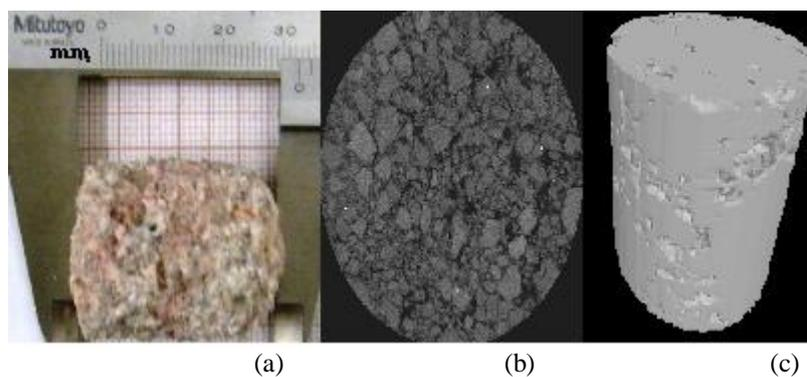
Figure 6: (a) The core at 2 m of depth. (b) One slice of 2-D  $\mu$ -CT visualization (c) 3-D  $\mu$ -CT image with 14.9  $\mu$ m of voxel resolution
