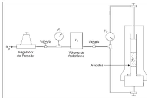
Figure 2: Scheme of Ultra poro-perm operation.
