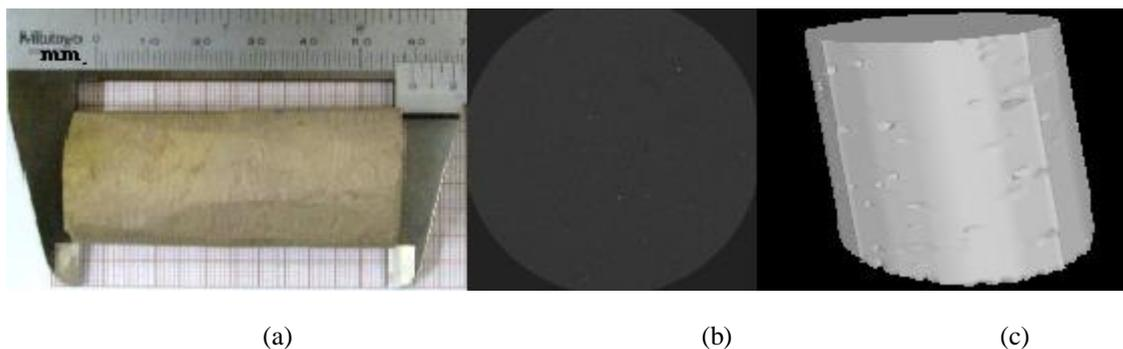
Figure 7: (a) The core at 6 m of depth. (b) One slice of 2-D  $\mu$ -CT visualization (c) 3-D  $\mu$ -CT image with 14.9  $\mu$ m of voxel resolution
