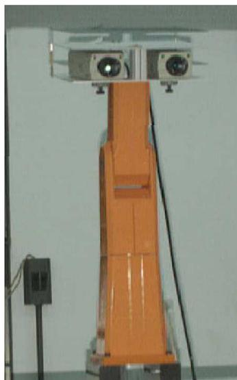
Figure 2. Vision system of the Janus robot.
