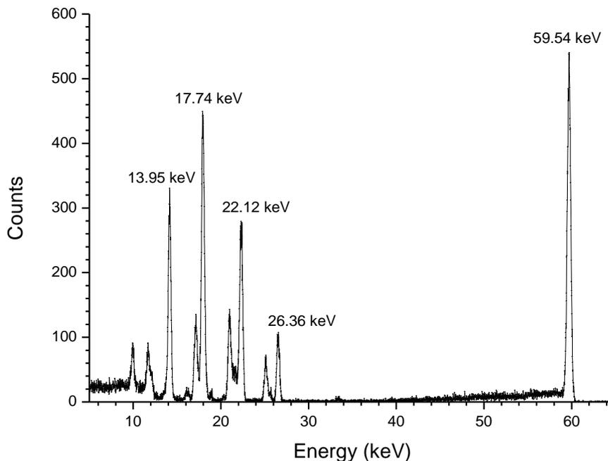
Figure 4. Spectrum Am-241 source non-sealed.
