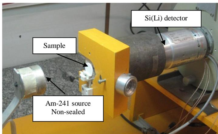
Figure 3. Picture of the experimental set-up of the method of transmission.
