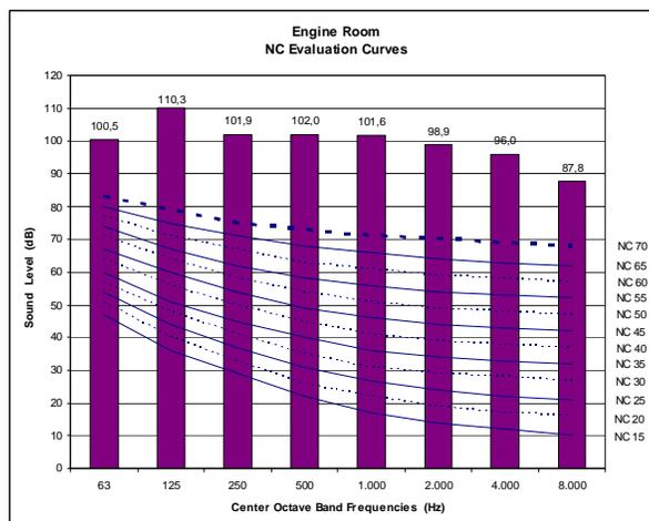
Figure 6. Octave band spectra of the sound level in the engine room superposed to the NC curves from NBR 10152:1987.
