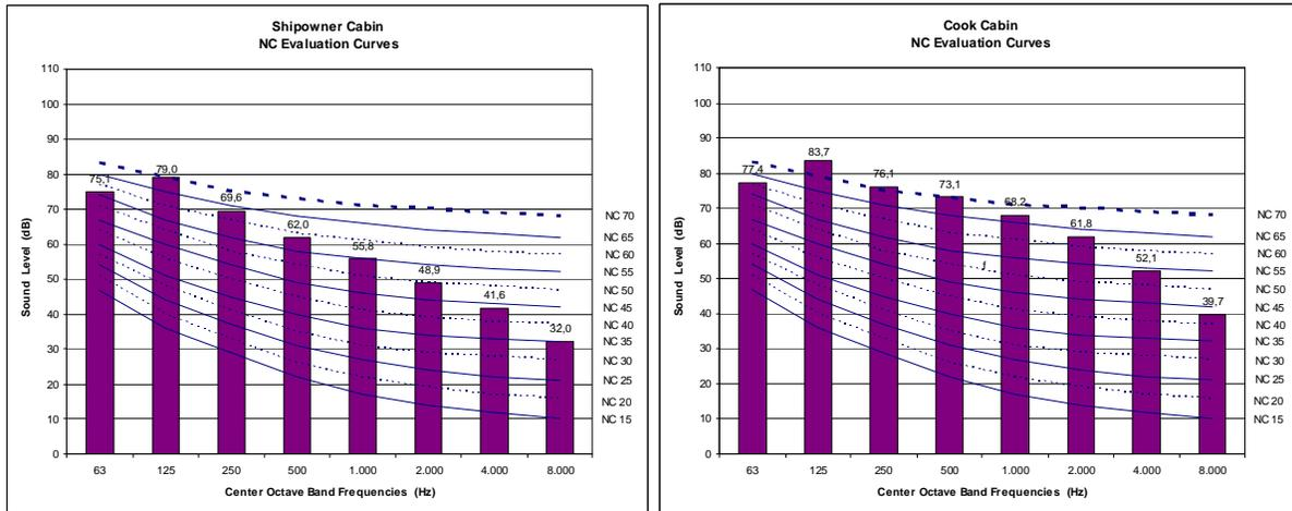
Figure 4. Octave band spectra of the sound level in the shipowner cabin and in the cook cabin, superposed to the NC curves from NBR 10152:1987.
