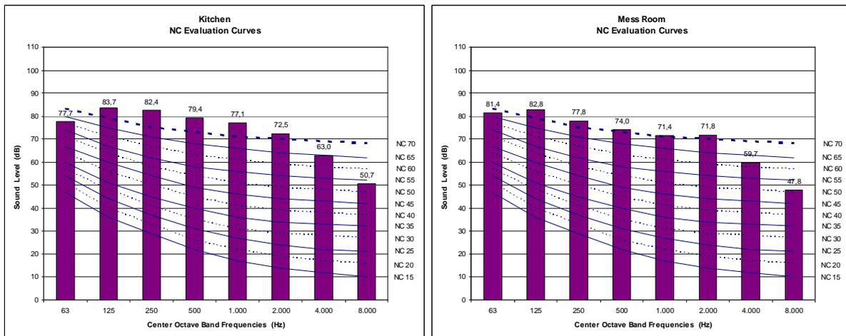
Figure 5. Octave band spectra of the sound level in the kitchen and in the mess room superposed to the NC curves from NBR 10152:1987.
